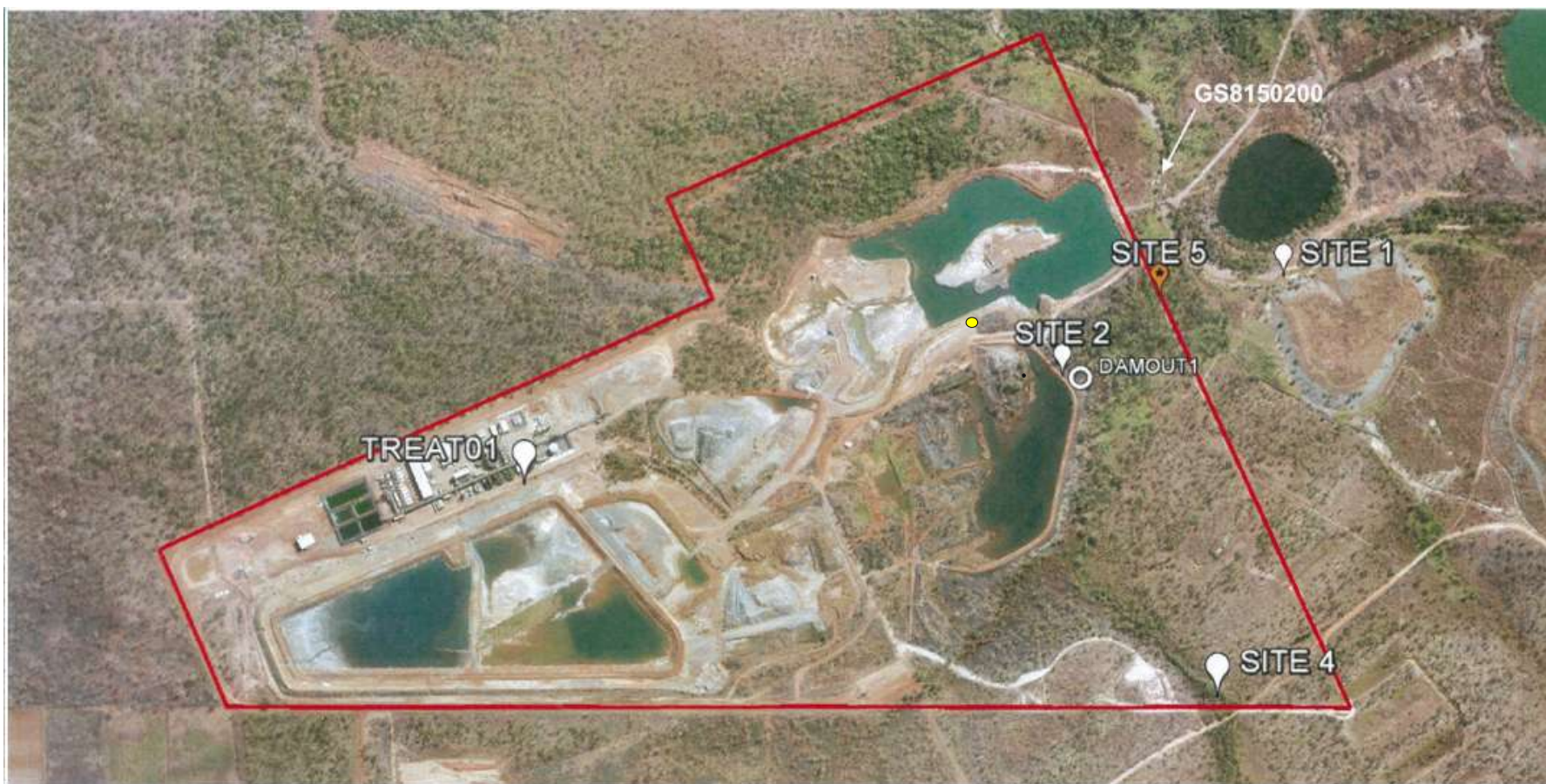
Figure 2 Site layout and surface water sampling sites (DAMOUT1 is the controlled discharge outlet from the Main Sediment Dam)
