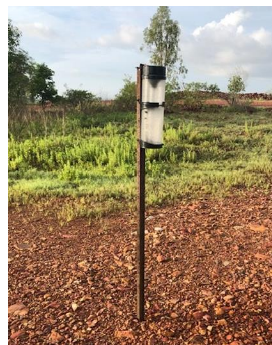
Rain gauge located at the top of the main WRD, Rustlers Roost
