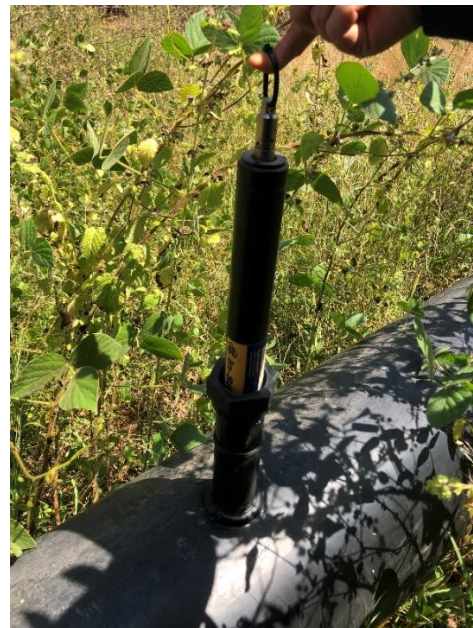
In-situ Aqua Troll sonde in housing end of pipe, water discharge from Rustlers Roost Pit, February 2022, Rustlers Roost PA
