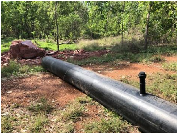
In-situ Aqua Troll sonde housing vertical in end of pipe, water discharge from Rustlers Roost Pit, January 2022, Rustlers Roost PA
