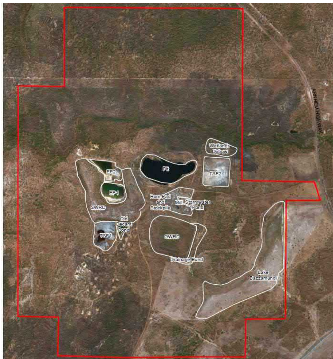
Figure 1 Layout of existing infrastructure. SWRD = Sulfide WRD; OWRD = Oxide WRD. Source: Supplement Appendix A
