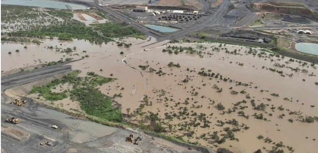
Looking north – flooding cut access between the Open Pit and Northern Overburden Emplacement Facility.
