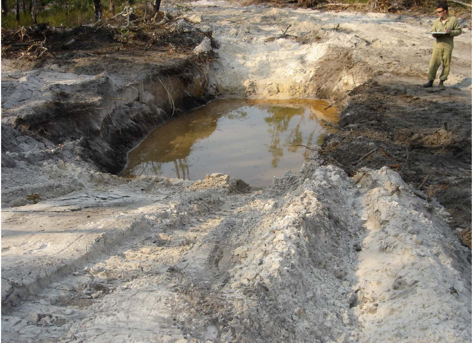
Larval Site 10 – Test pit in Andranangoo Creek West prospect area. Note the pit had been excavated to below the ground water table. Looking north.
