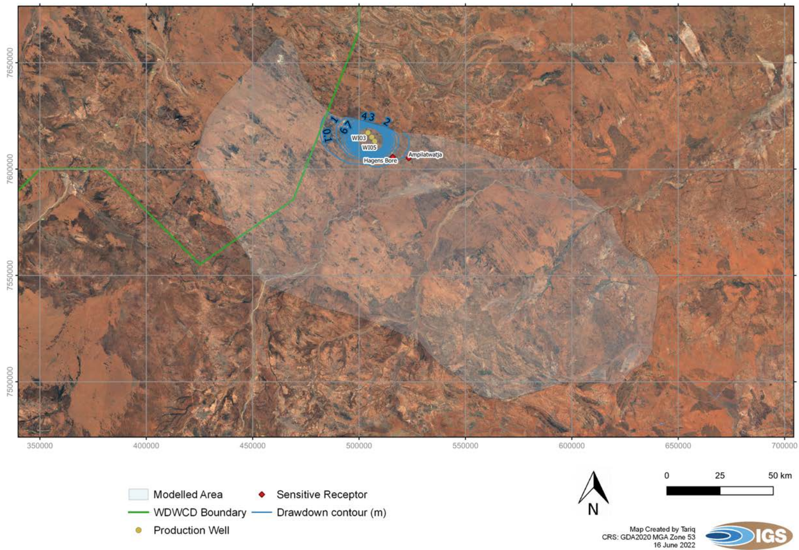
Figure 30. WDWCD flux P10 drawdown contours at the end of 25-year operation.
