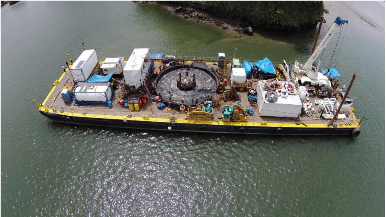
Figure 2-51. Example of cable lay barge (Source: Geomares)
