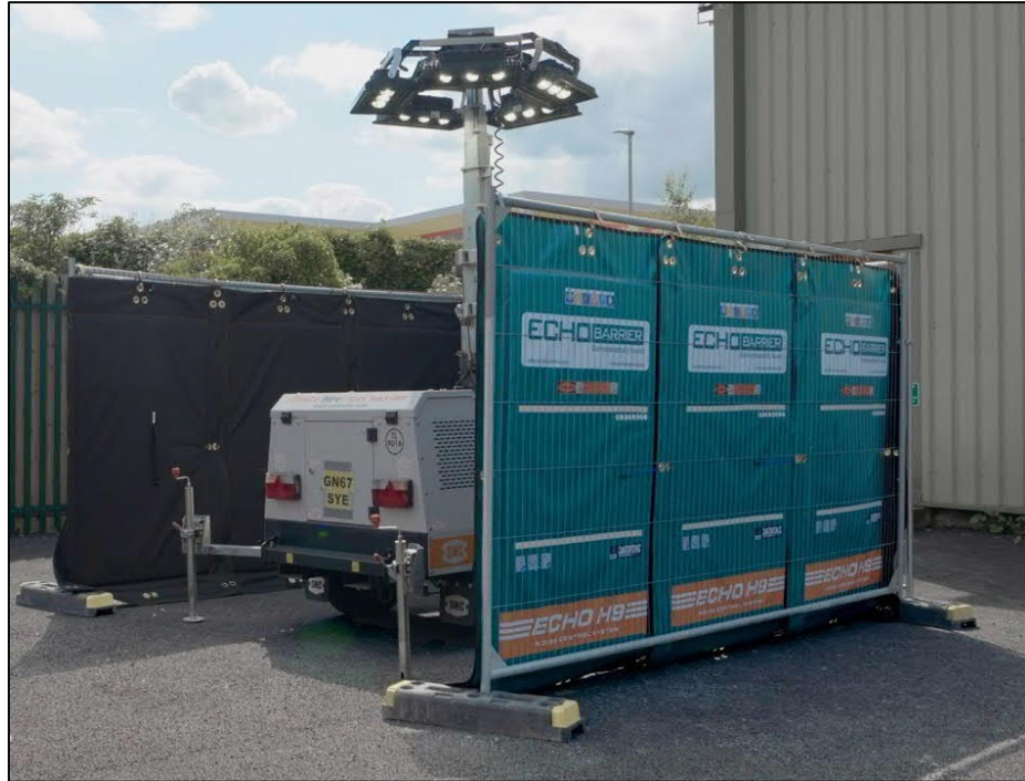
Figure 1-9: Temporary Noise Enclosure Example
