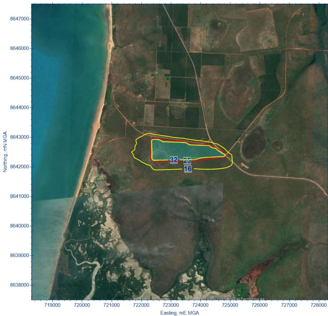
Figure 8-43 Predicted maximum cumulative 24-hour average PM_{2.5} concentration for the Darwin Converter Site
