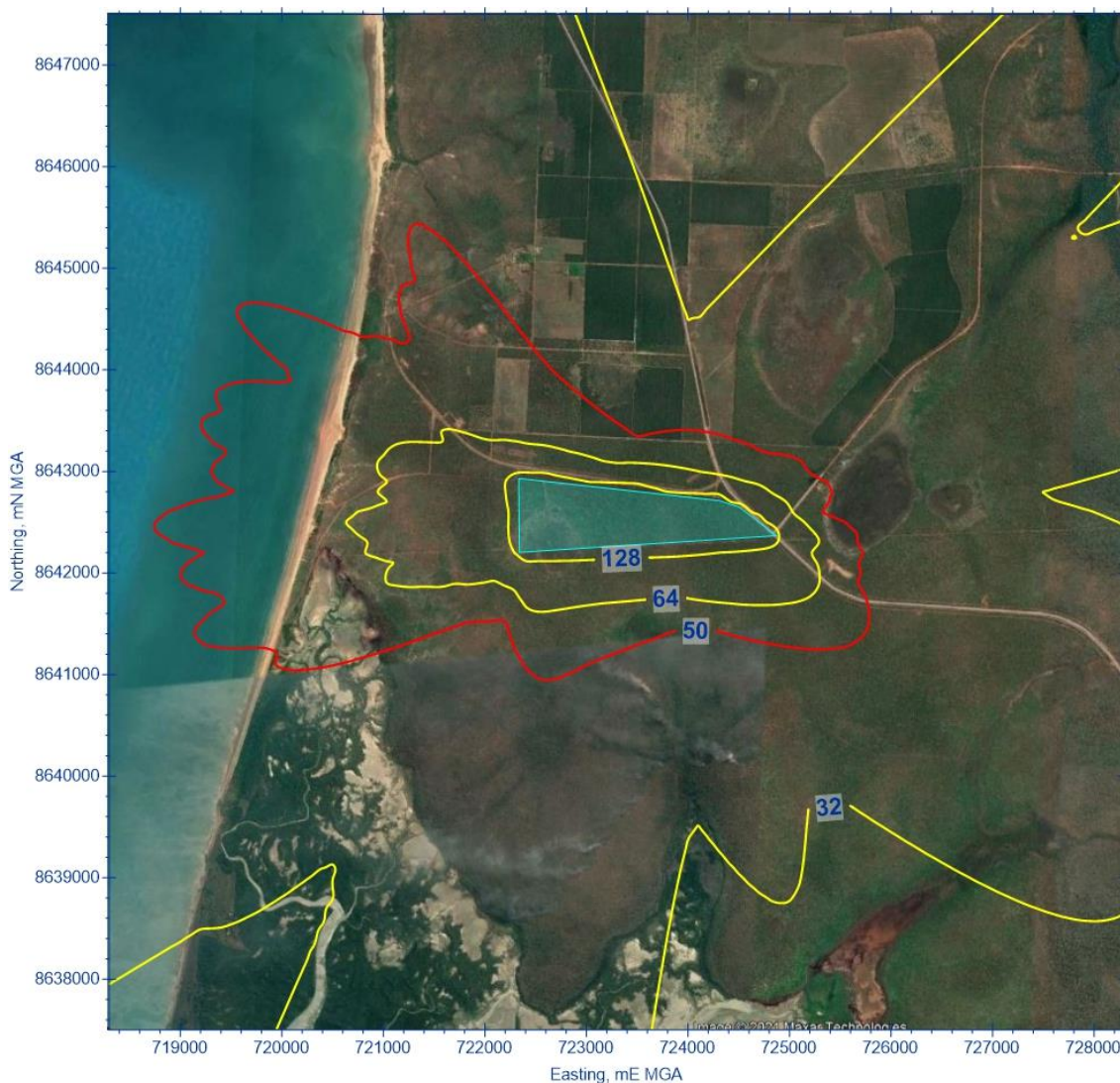
Figure 8-47 Predicted maximum cumulative 24-hour average PM_{10} concentration for the Darwin Converter Site
