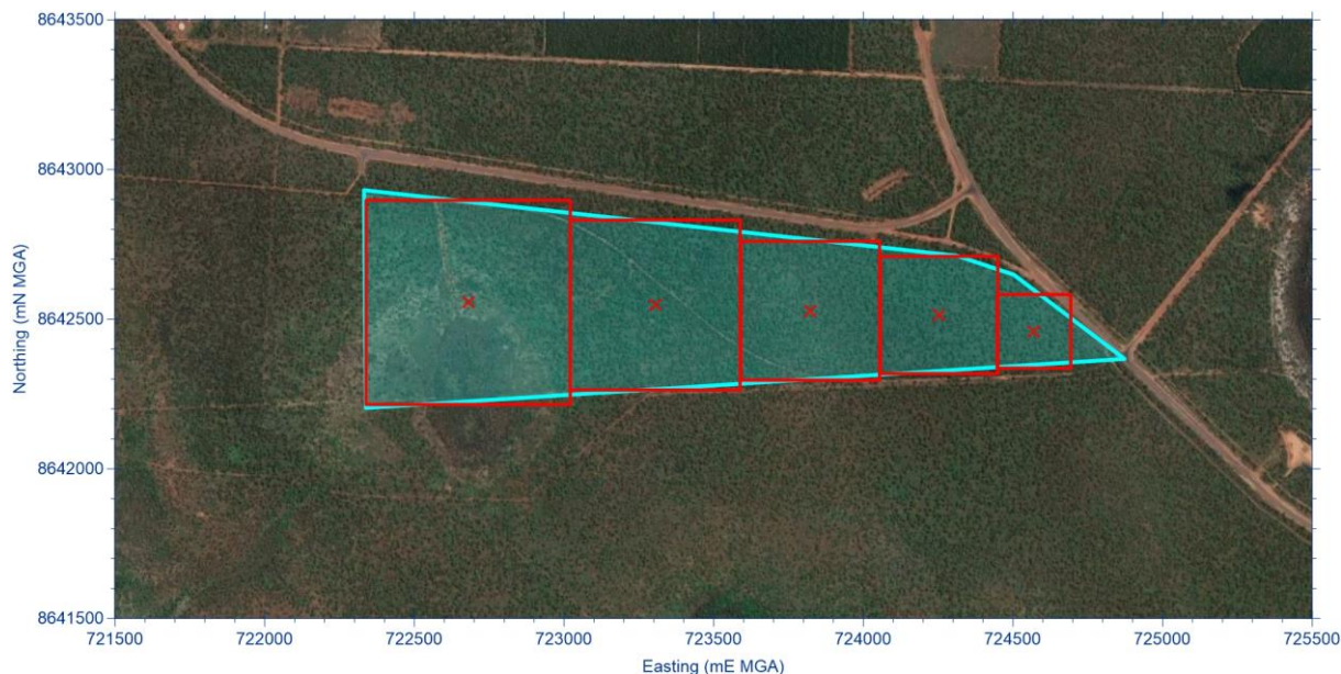
Figure 4-2 Location and extent of the five volume sources representing diesel emissions from construction vehicles at the Darwin Converter Site
