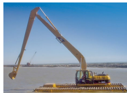
CAT amphibious excavator – extended arm (12m, 15m, 18m, 22m reach)
