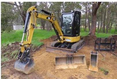
3.5 T CAT excavator on tracks (different accessories) for primary channels
