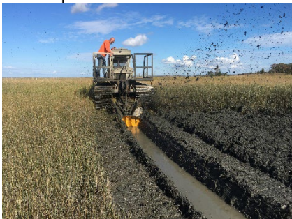
MarshMaster – different design to an excavator
