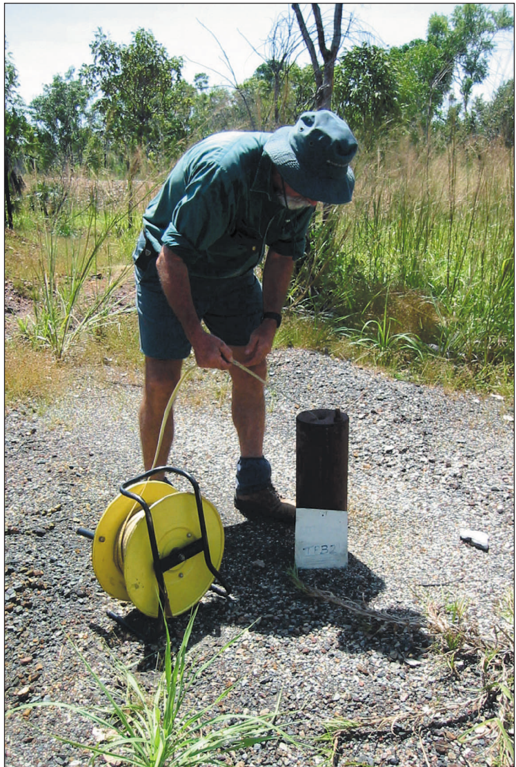
Plate 7.8 Groundwater borehole monitoring near the trial pit
