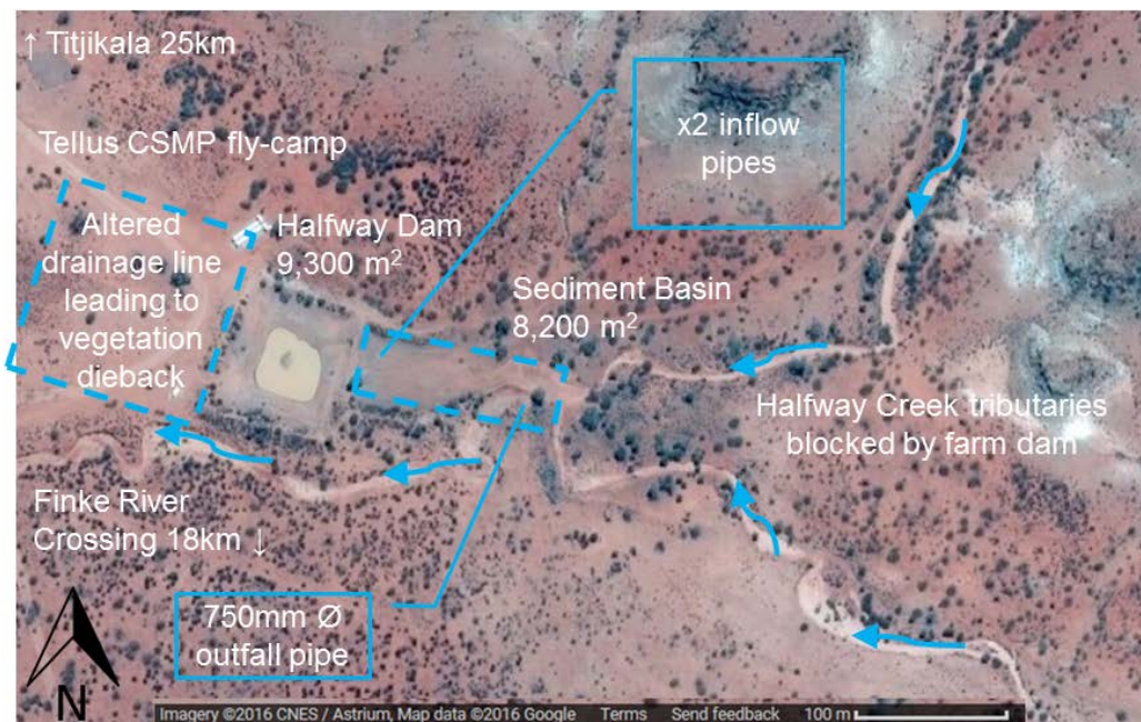
Figure 9-14 Hydraulic characteristics of Halfway Dam
