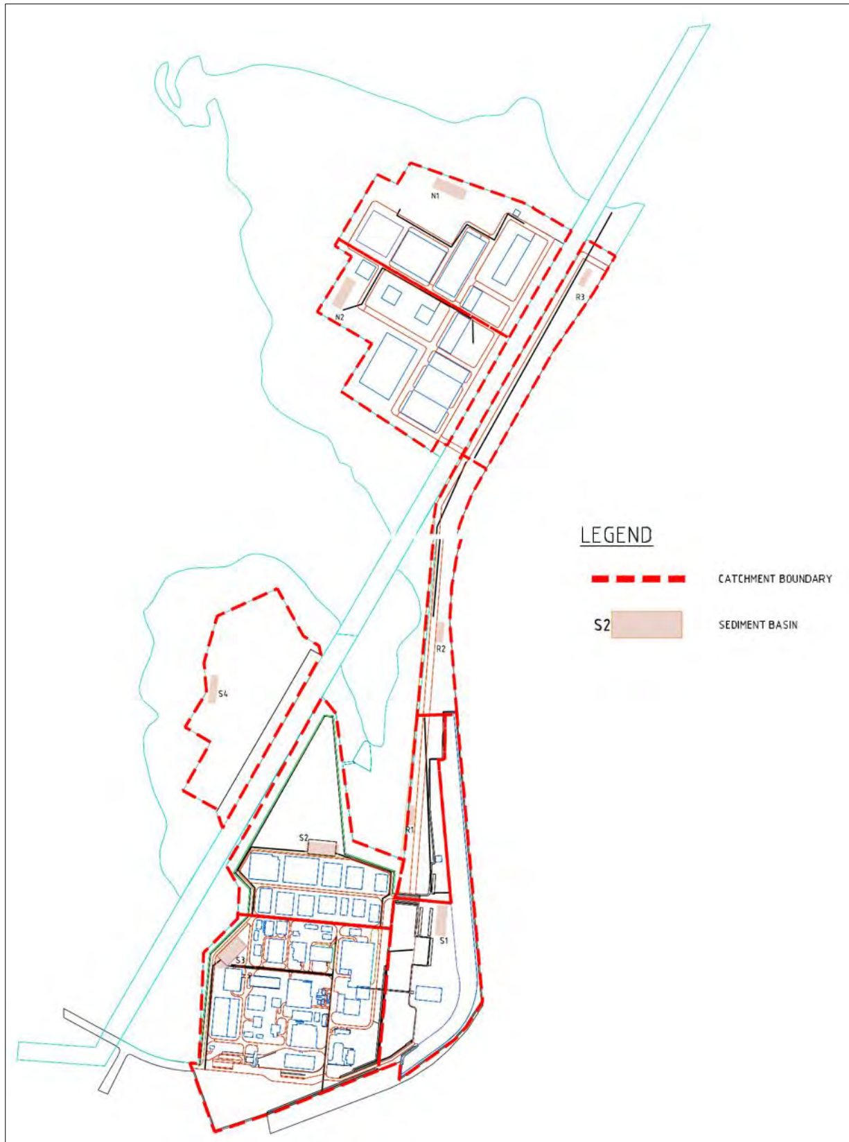
Figure 2-5. Catchments and basins in the Development Envelope
