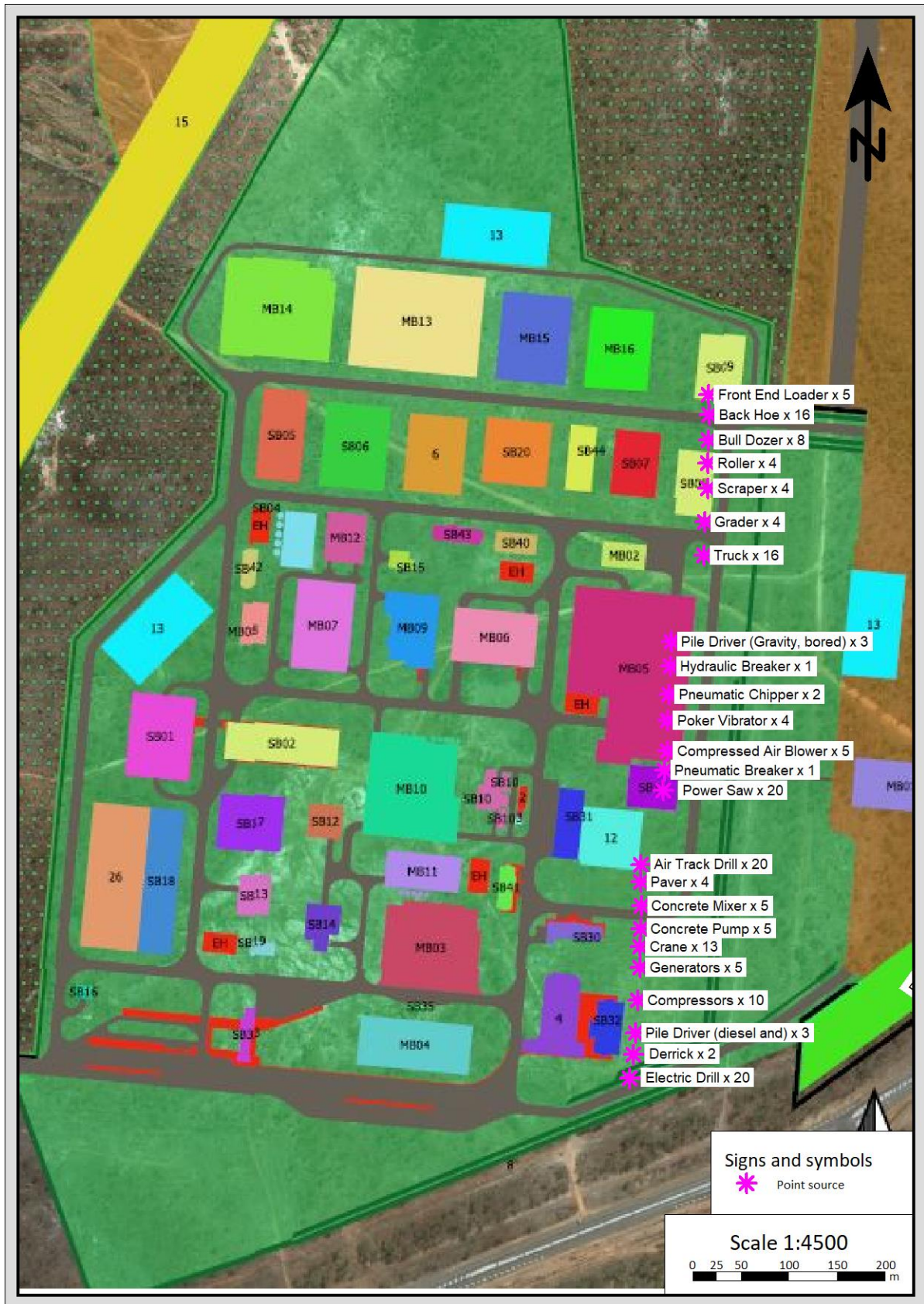
Figure 6-2: Location of Noise Sources – Construction – South
