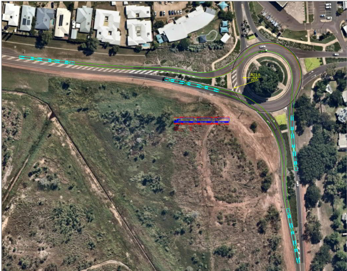
Figure 20 Sketch of the Kirkland Road / Elrundie Roundabout turning movement for a Triple Road Train
