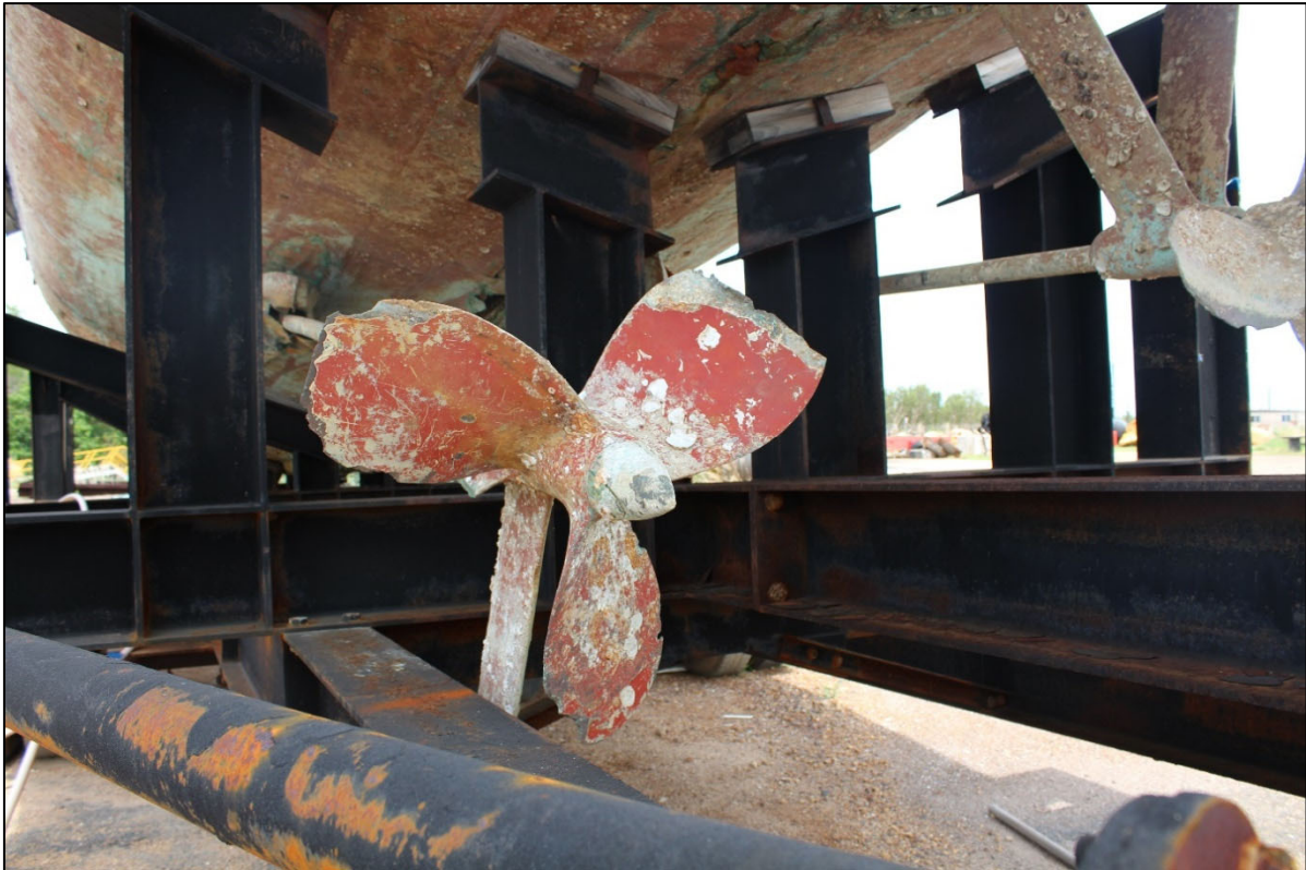
Figure 20: Port side propeller showing damage
