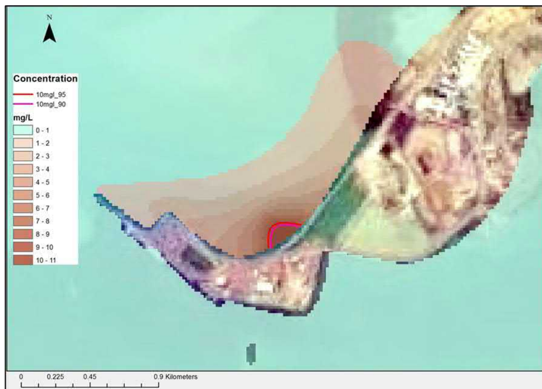
Figure 7-4 SSC (above background) outside the discharge location from the EAW settlement ponds showing the 90 th and 95 th percentile exceedance of 10 mg/L SSC
