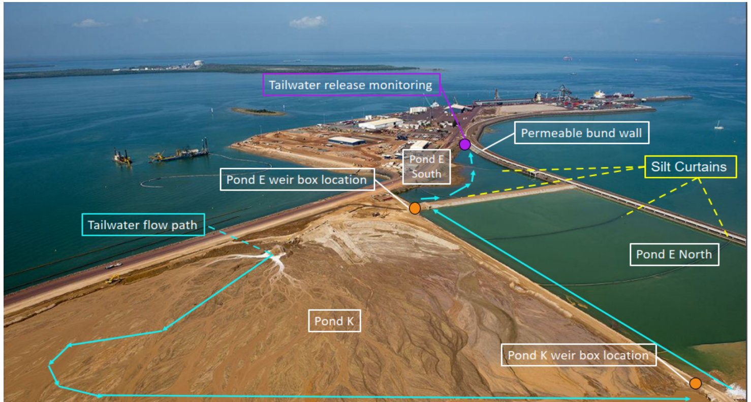
Figure 4 Proposed monitoring locations and tailwater flow based of the 2012 MSB dredging campaign
