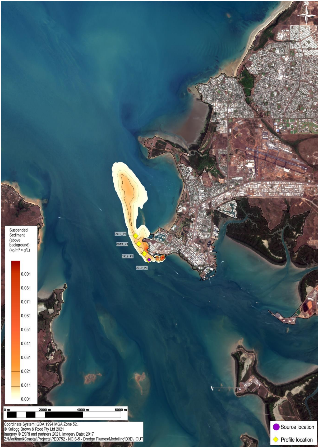
Figure B.3 Suspended sediment concentrations above background – Depth-averaged instantaneous result at 19/09/2013 08:30 with measured locations (with depth profile locations)
