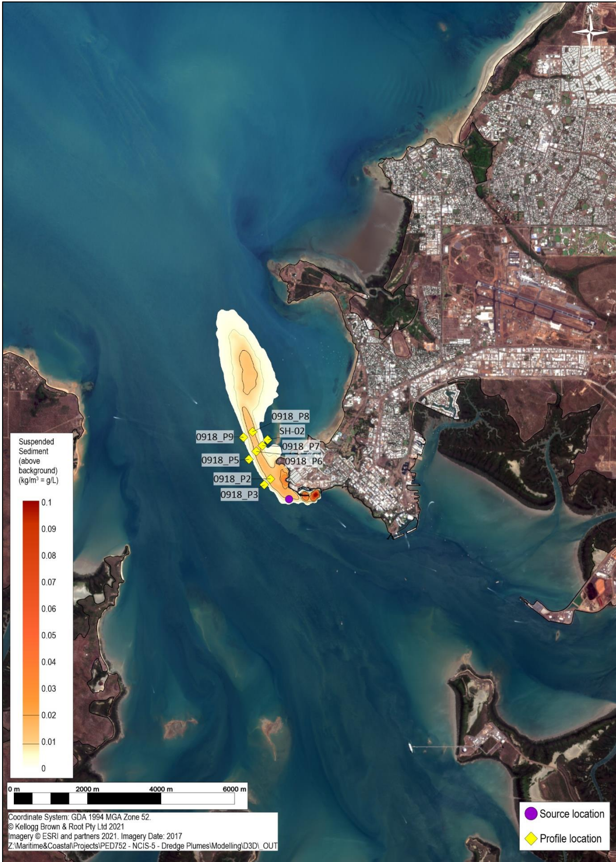
Figure B.1 Modelled suspended sediment concentrations above background – Depth-averaged instantaneous result at 18/09/2013 11:00 (with depth profile locations)
