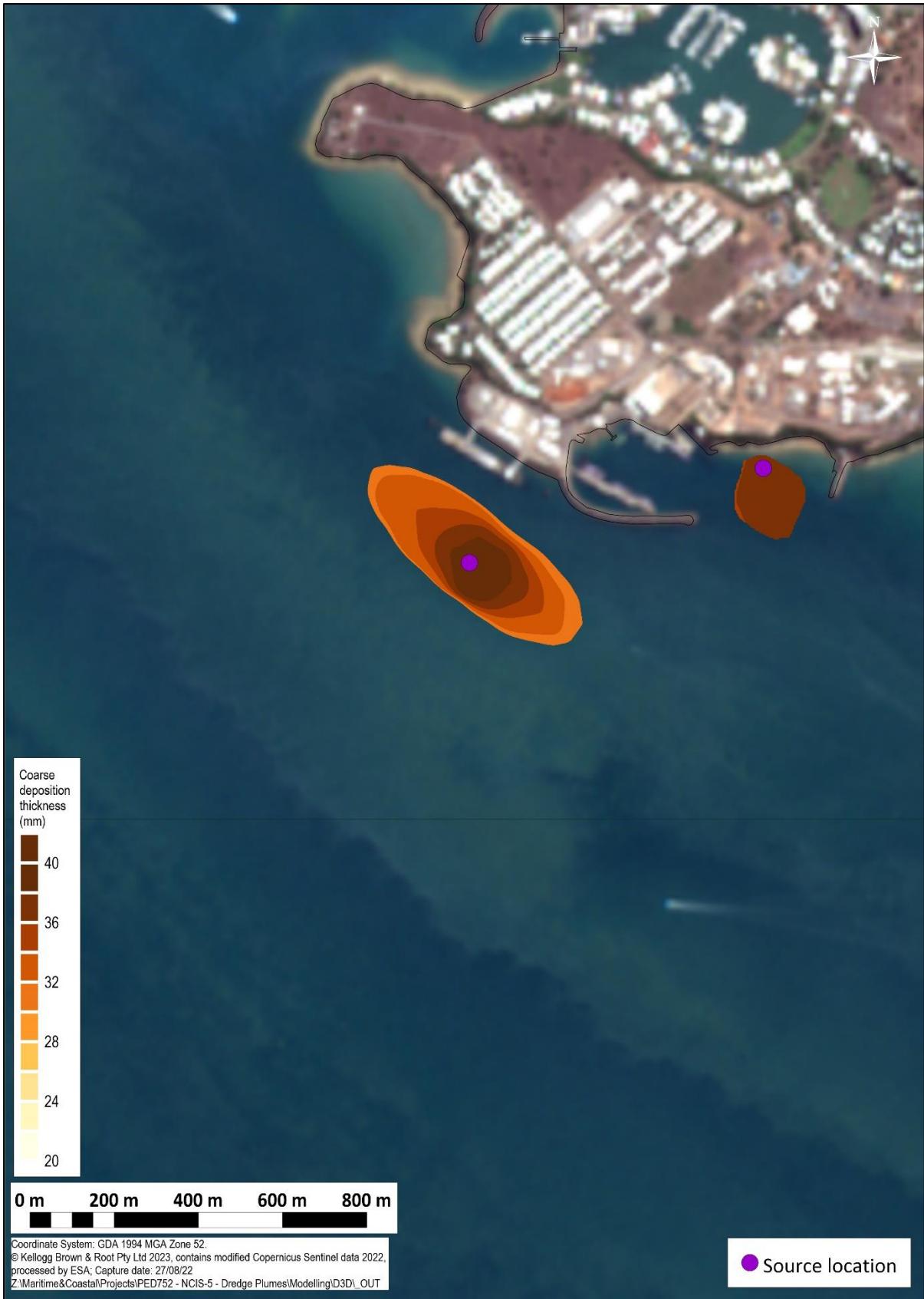
Figure 6.1 Zones of coarse deposition and thickness (mm)
