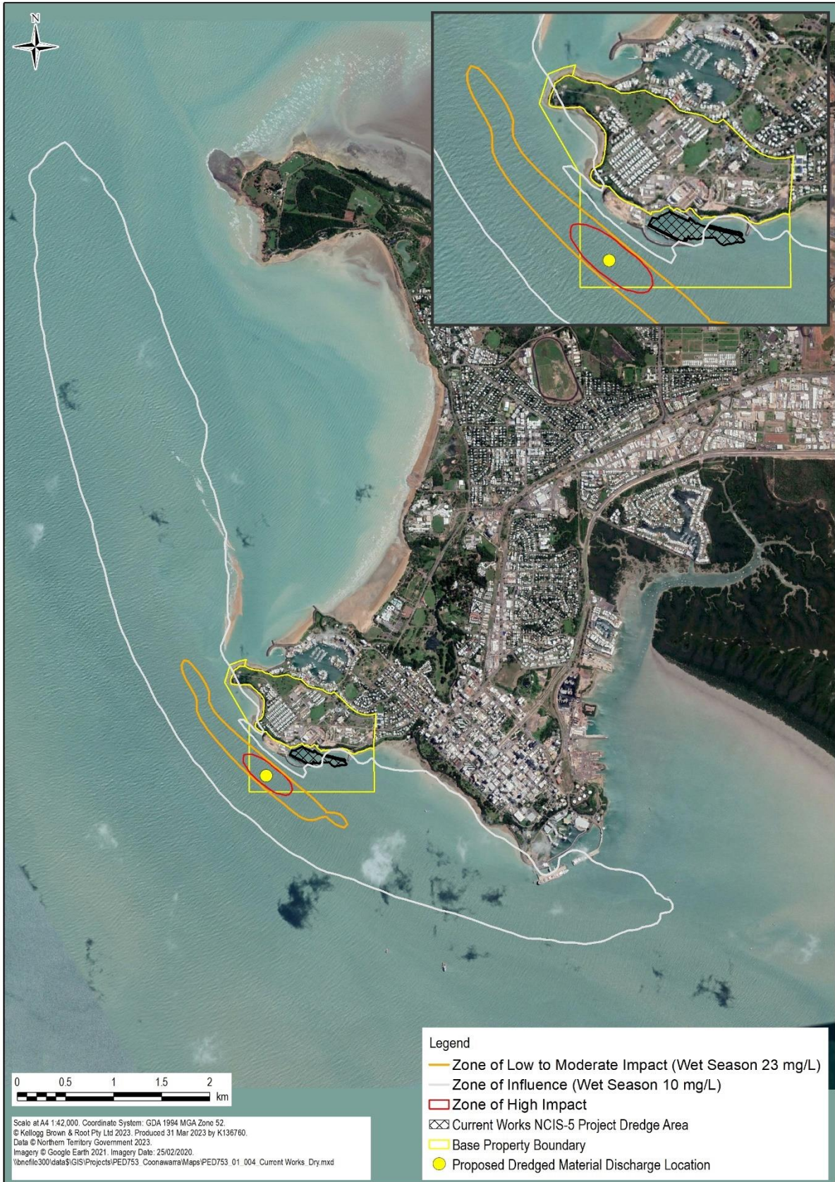
Figure 5.28 90 th percentile current NCIS-5 project suspended sediment concentration zones of impact and influence (Wet Season - includes 5 mg/L background)
