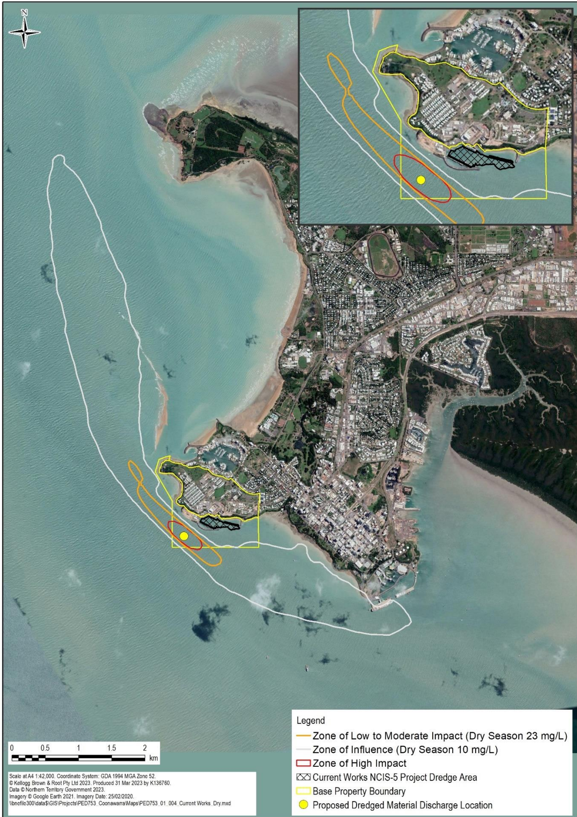
Figure 3.33 90th percentile current NCIS-5 project suspended sediment concentration – Zones of impact and influence (Includes 3 mg/L background – Dry Season)
