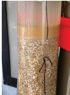
Figure 3: Settling of fine material from the water column on top of bed sediment
