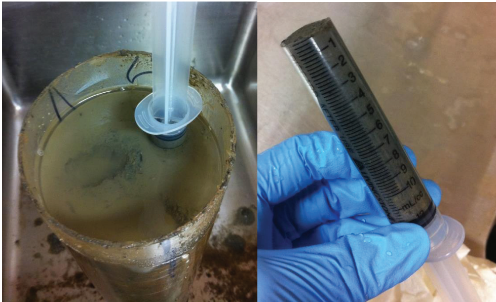
Figure 4: Taking core samples of known volume for bulk density testing
