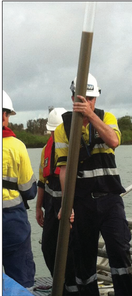
Figure 2: A core taken showing no distinction between the turbid water and the mud sample.
