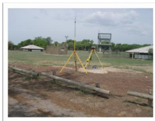
Figure 10 RTK GPS Reference Station
