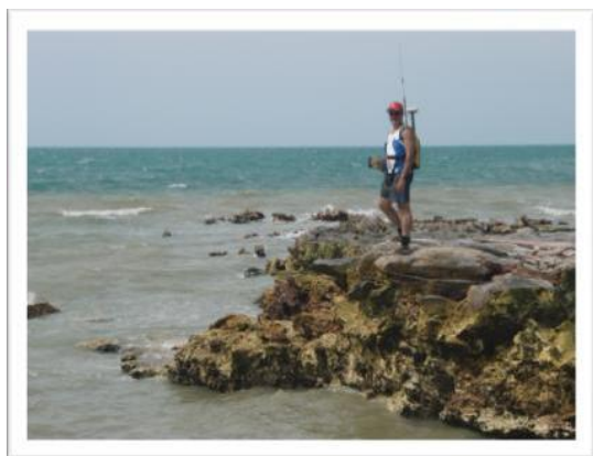
Figure 9 Backpack mounted RTK GPS.
