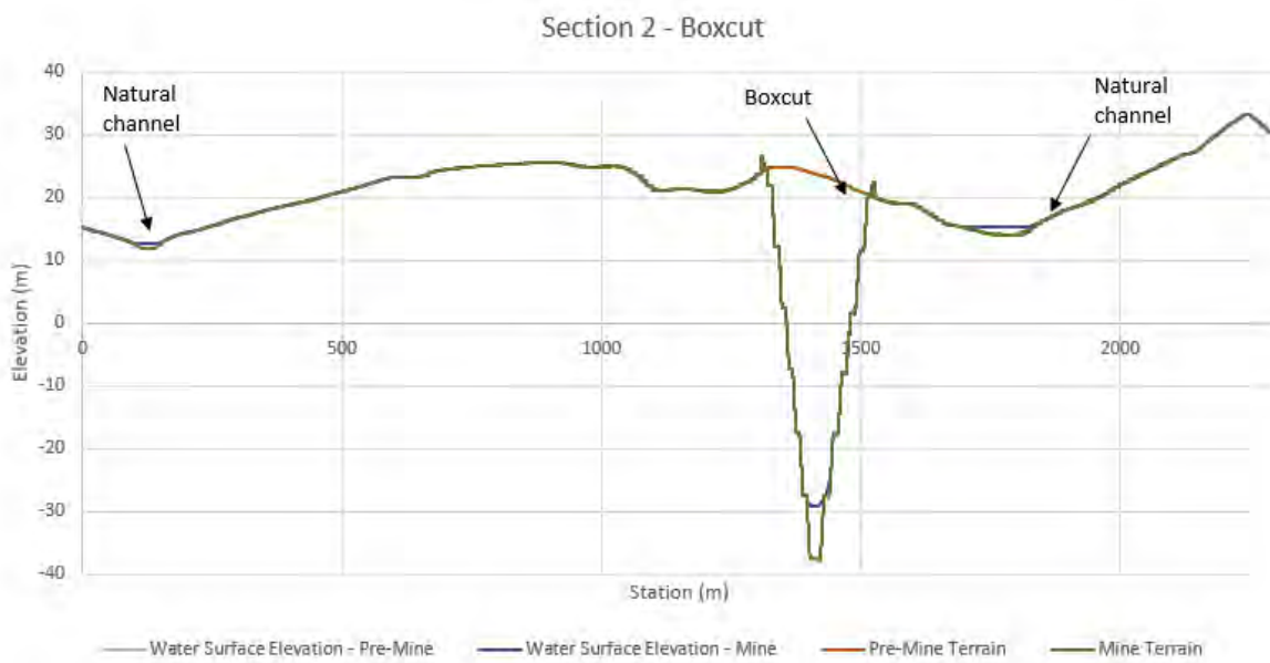
Figure 33. Cross-section 2 through boxcut showing pre-mine and mine scenario water depths for the 1%AEP event
