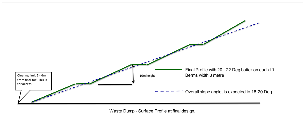
Figure 8: Cross-section of a typical construction and final slope profile for the proposed Elizabeth Marion waste rock landform
