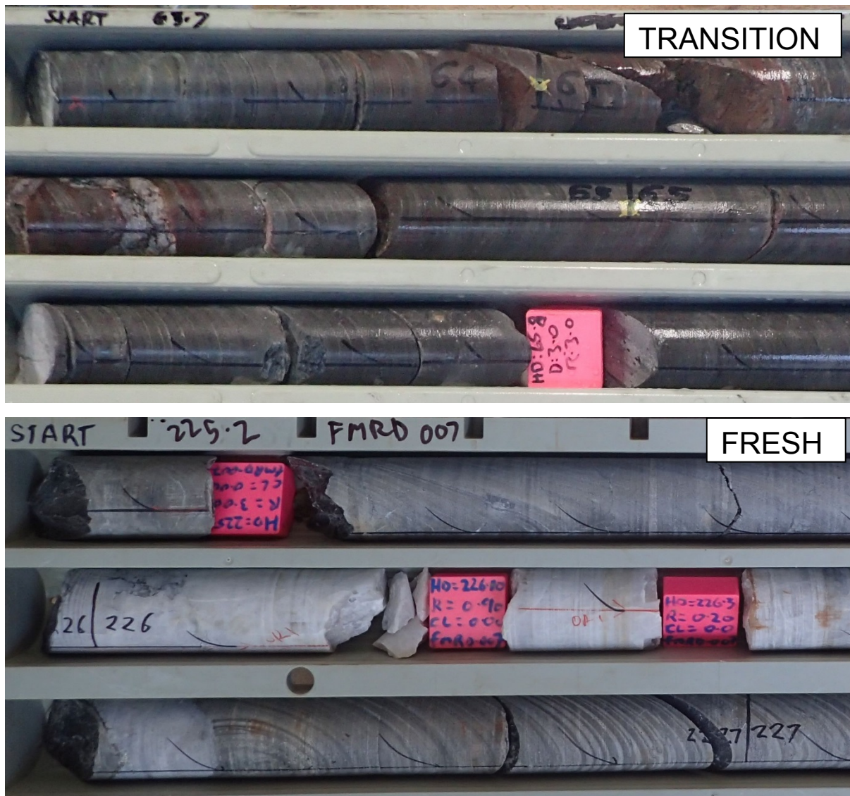
Figure H Photographs of the three weathering domains of Quartz Veins from Grants (Top = Weathered, Middle = Transitional, Bottom = Fresh)
