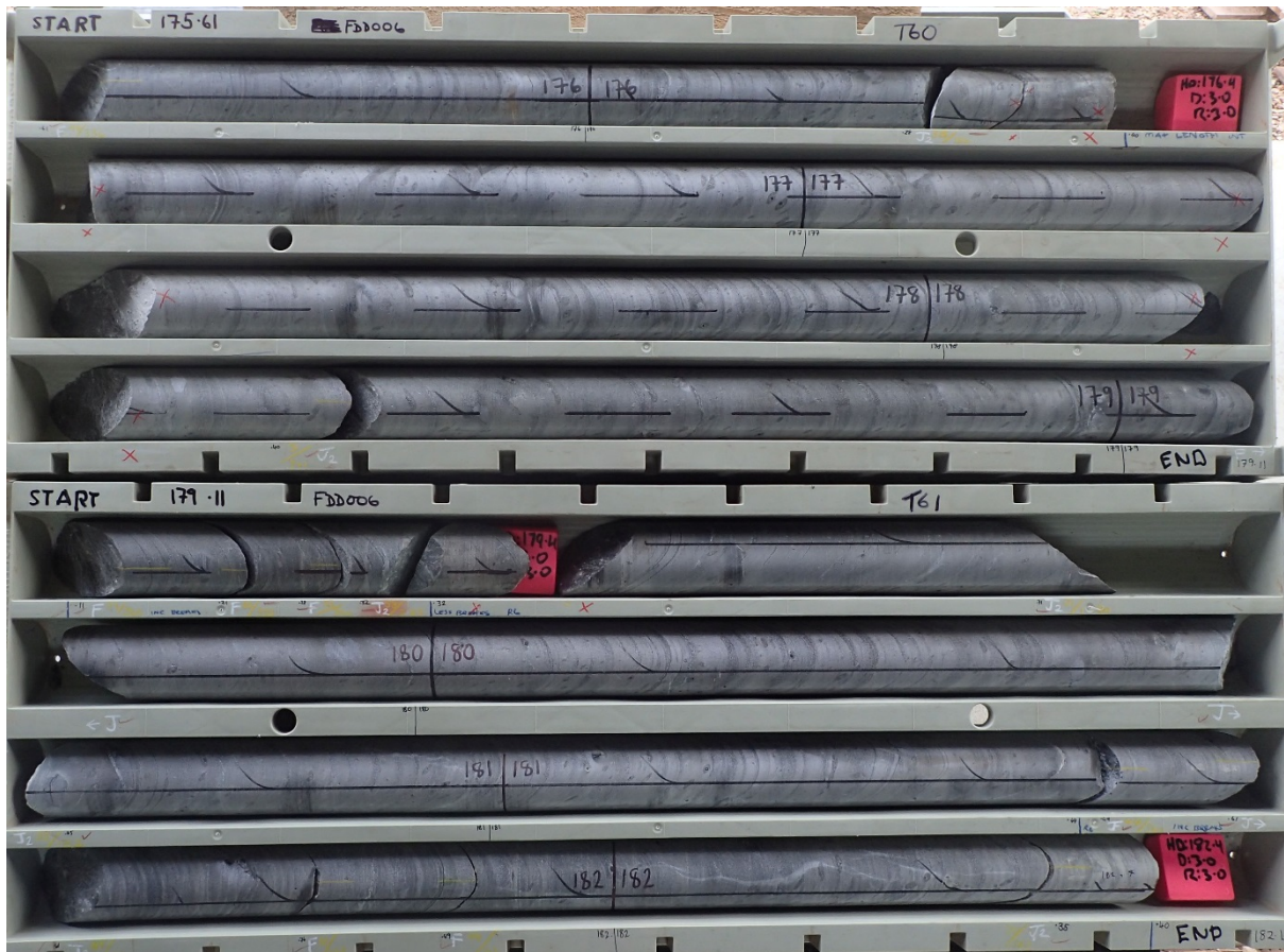
Photograph of typical intersection of Burrell Creek Formation Fresh phyllite from Grants (FMRD006, 175-182m).
