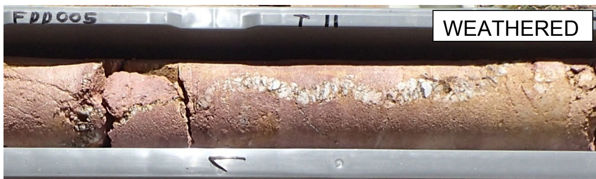
Photographs of the three weathering domains of BCF phyllite from Grants (Top = Weathered, Middle = Transitional, Bottom = Fresh)
