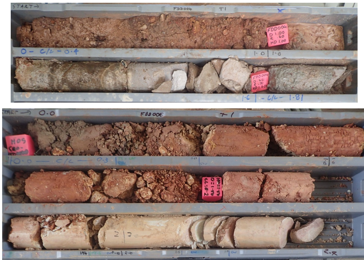
Figure 3-1. Photographs showing typical soil and soil-laterite profiles from Grants
