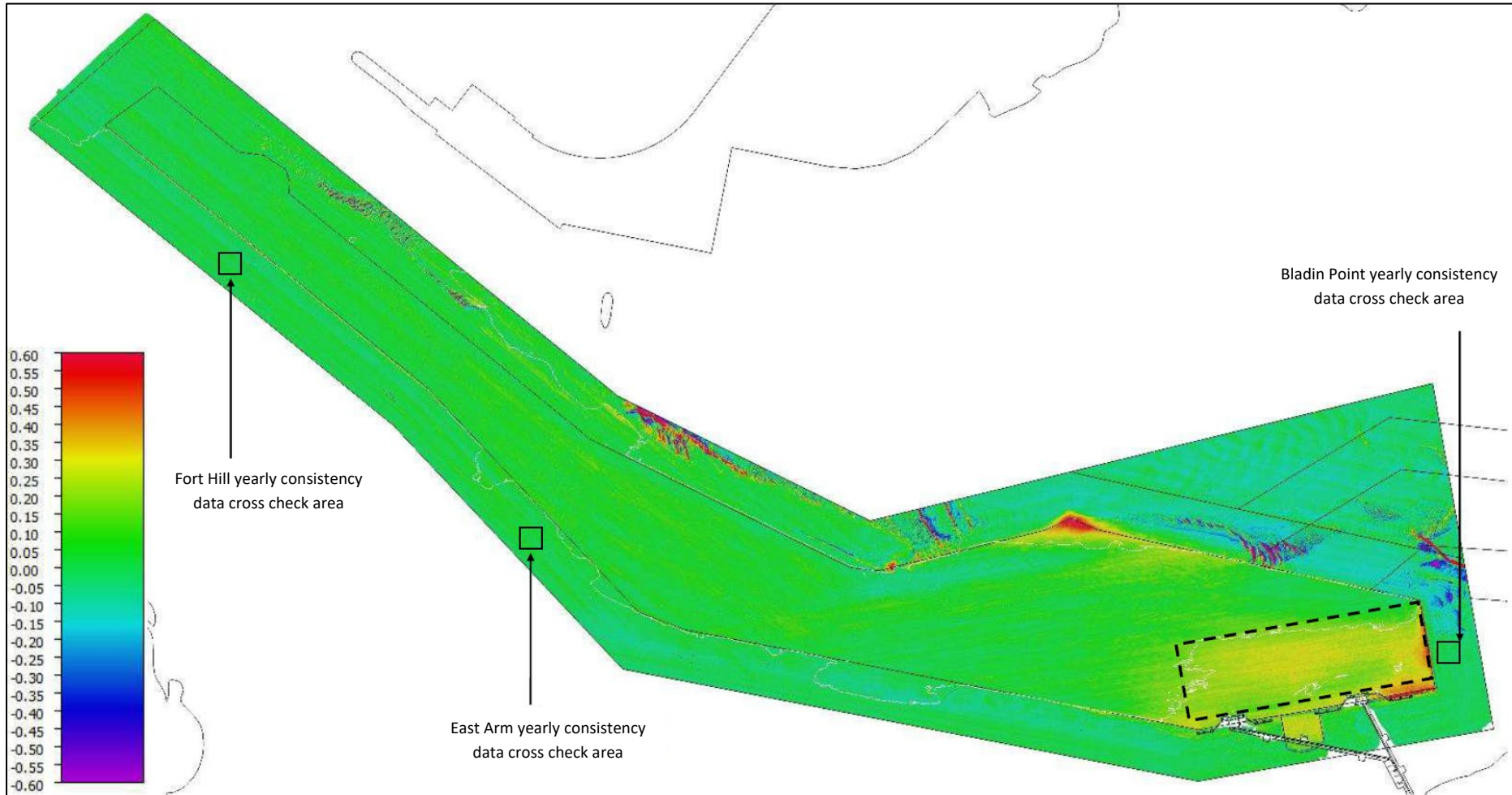
Figure 1: Dredge area surface difference 2018 (+) compared to 2017 (-). Depth contour -13.5m LAT shown (white). Mean surface difference of +22 cm in black dashed area.
