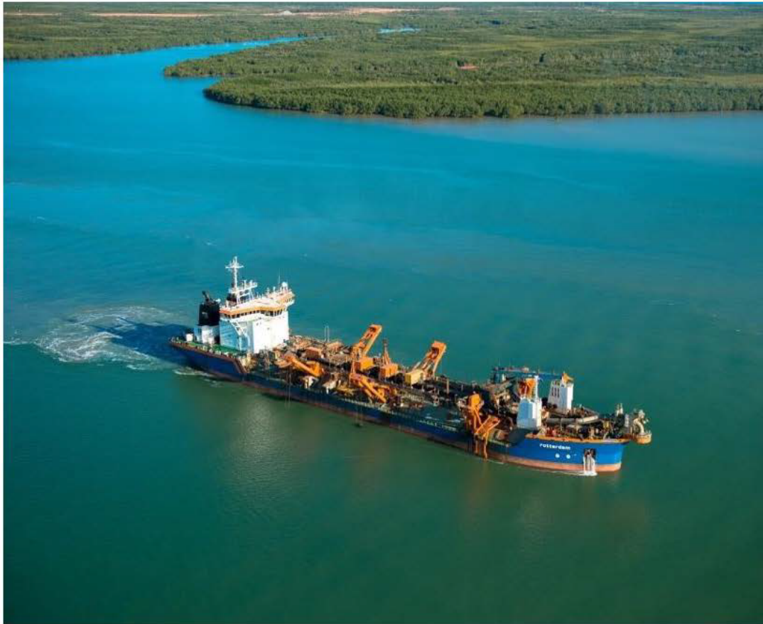
Figure 2: Trailing suction hopper dredge.
