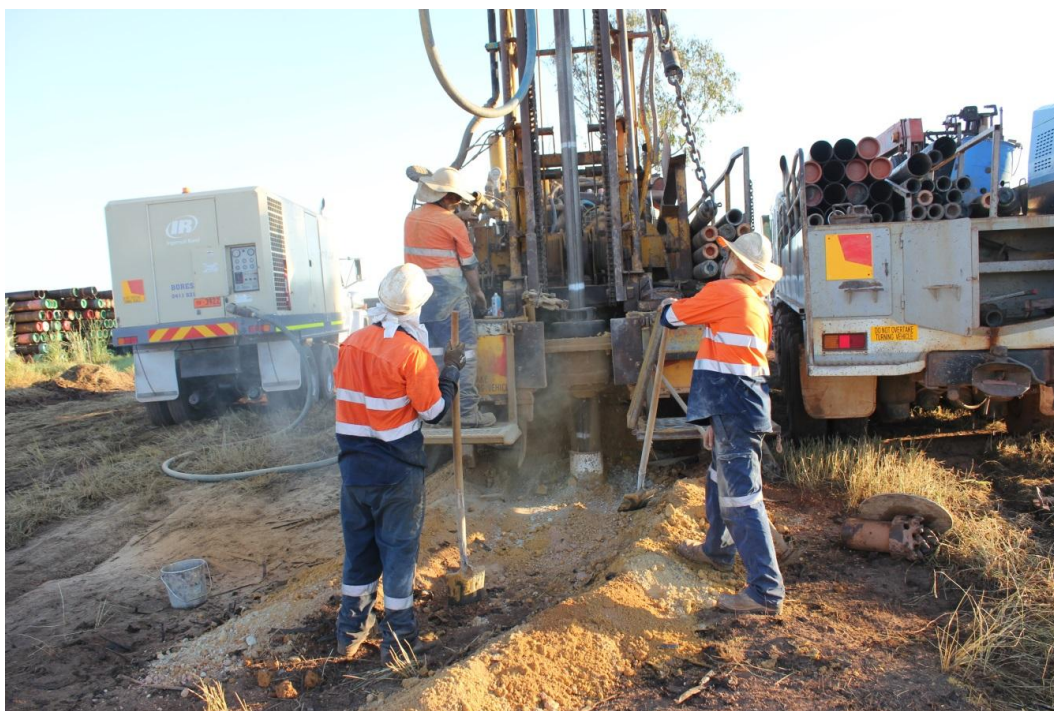
Figure 3 Rotary Air Blast Drilling (Note 1m marks on drill stem for sampling)
