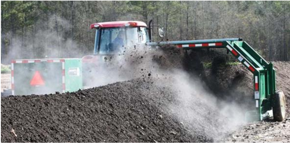
Figure 21 A Tractor Drawn Windrow Turner Turns the Compost
