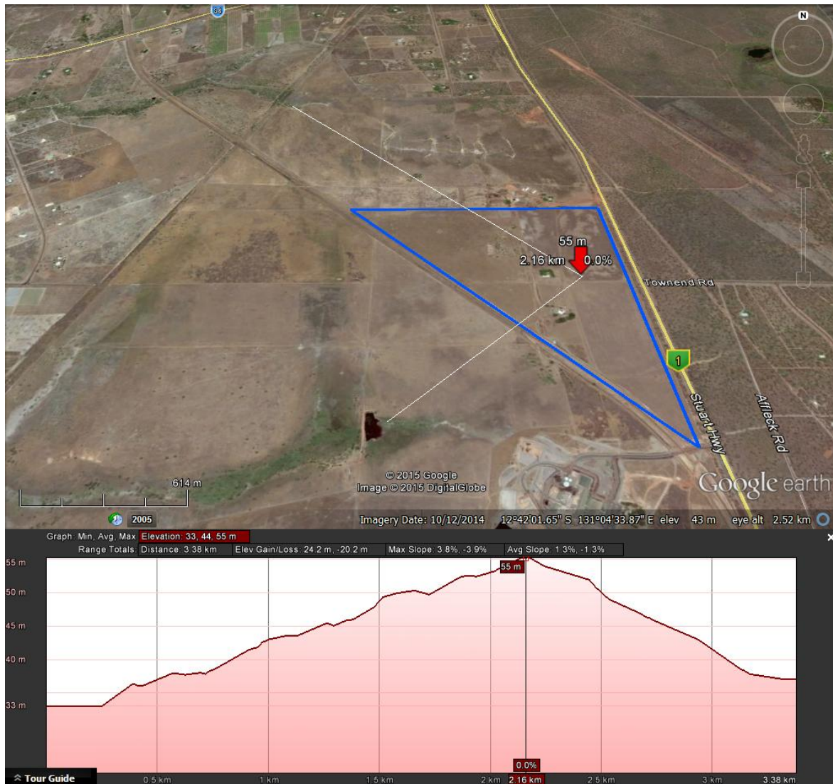
Figure 2 Topographic Cross section plan from irrigation area midpoint to nearest watercourses
