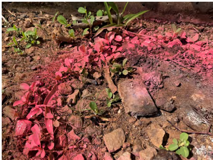
Photo 21 Northern perimeter, external wall, ACM fragment marked in pink
