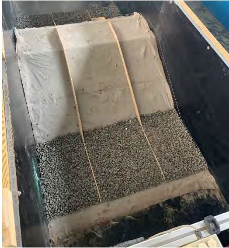
(g) Core box lined with geotextile and quarry run on the leeside and seaside toes
