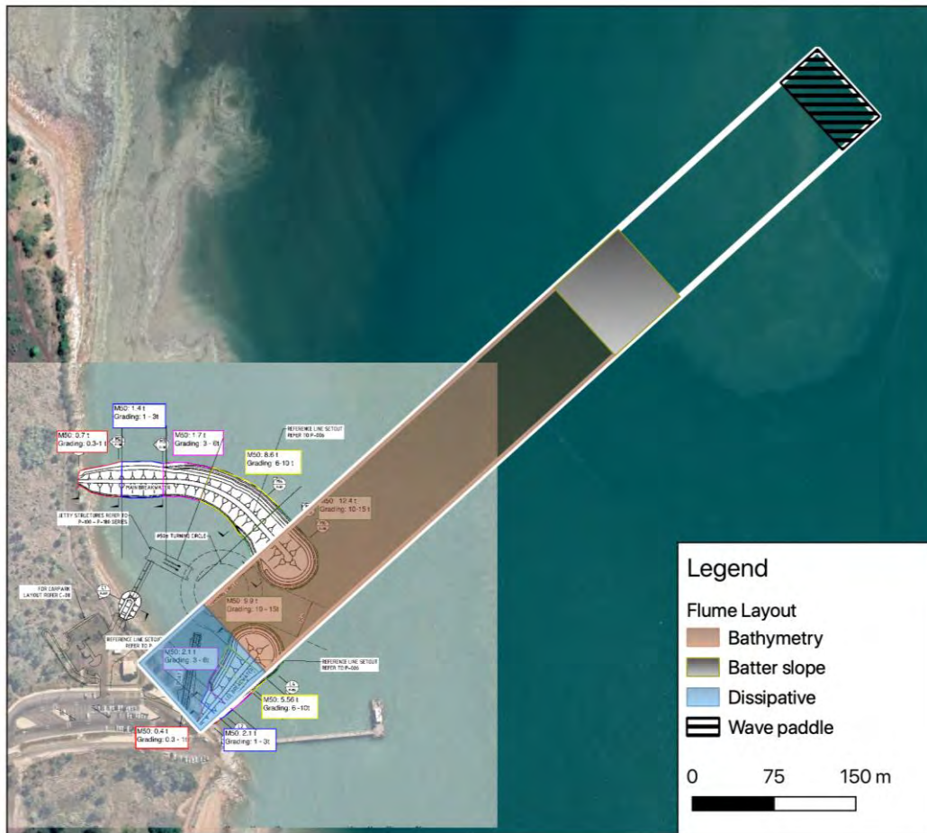
Figure 4.3 Overview of the bathymetry built in the wave flume relative to project site
