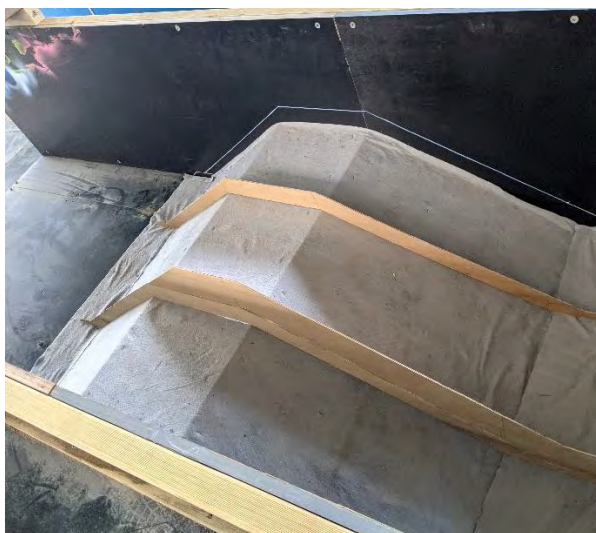
(a) Core box lined with geotextile
