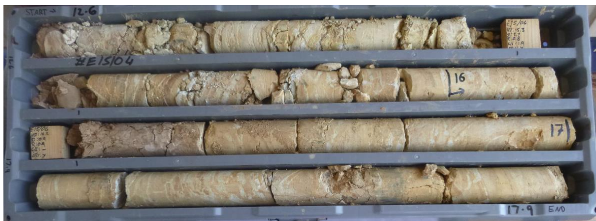
Figure 8-8 Tray 4 (12.6-17.6 m) Transition to Weathered Bleached HYC Shale Bedrock with Lenses of Silts and Sands
