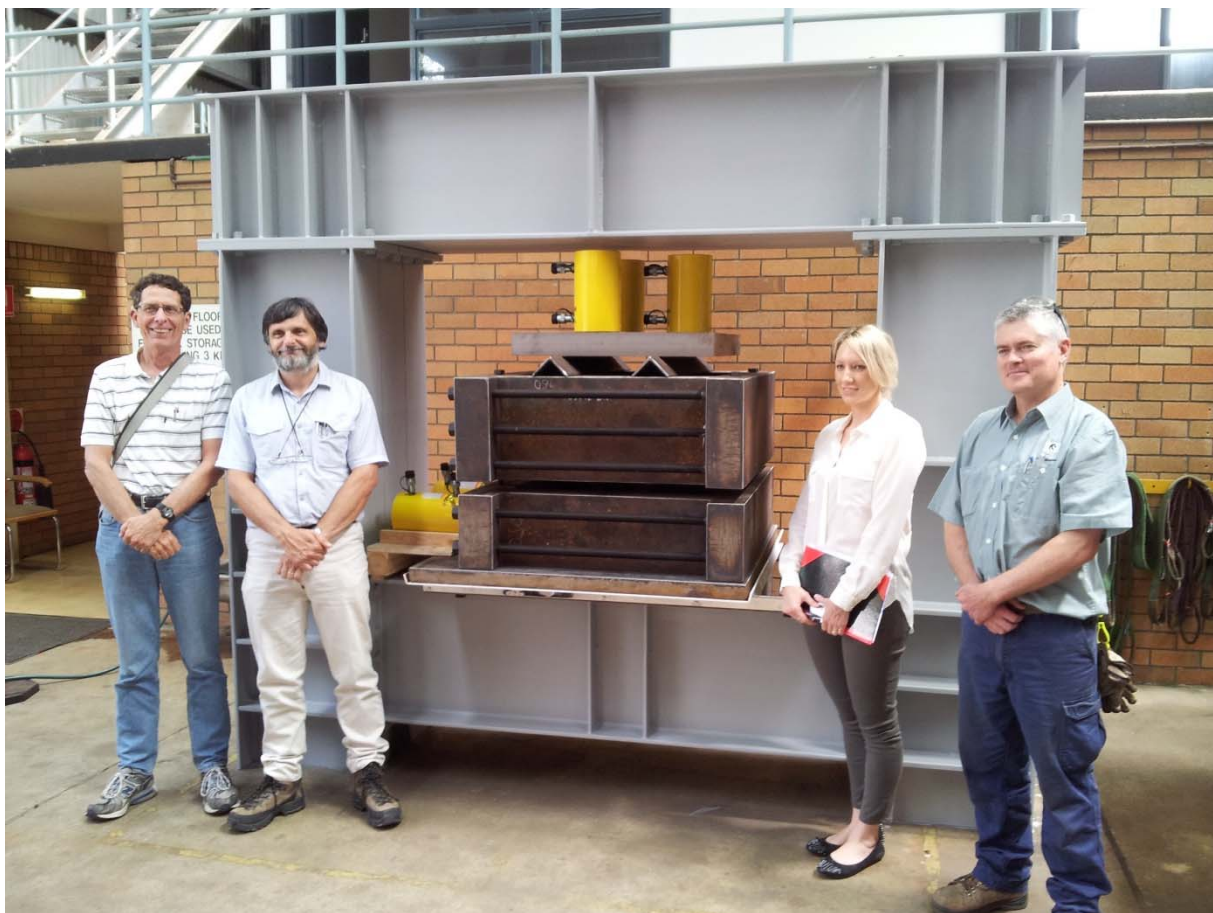
Figure 6 UN’s large-sized direct shear testing machine
