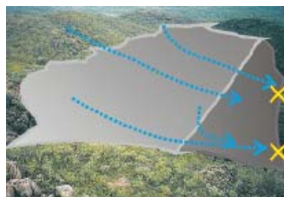
Figure 6 - water table ‘moving’ into the waste facility
