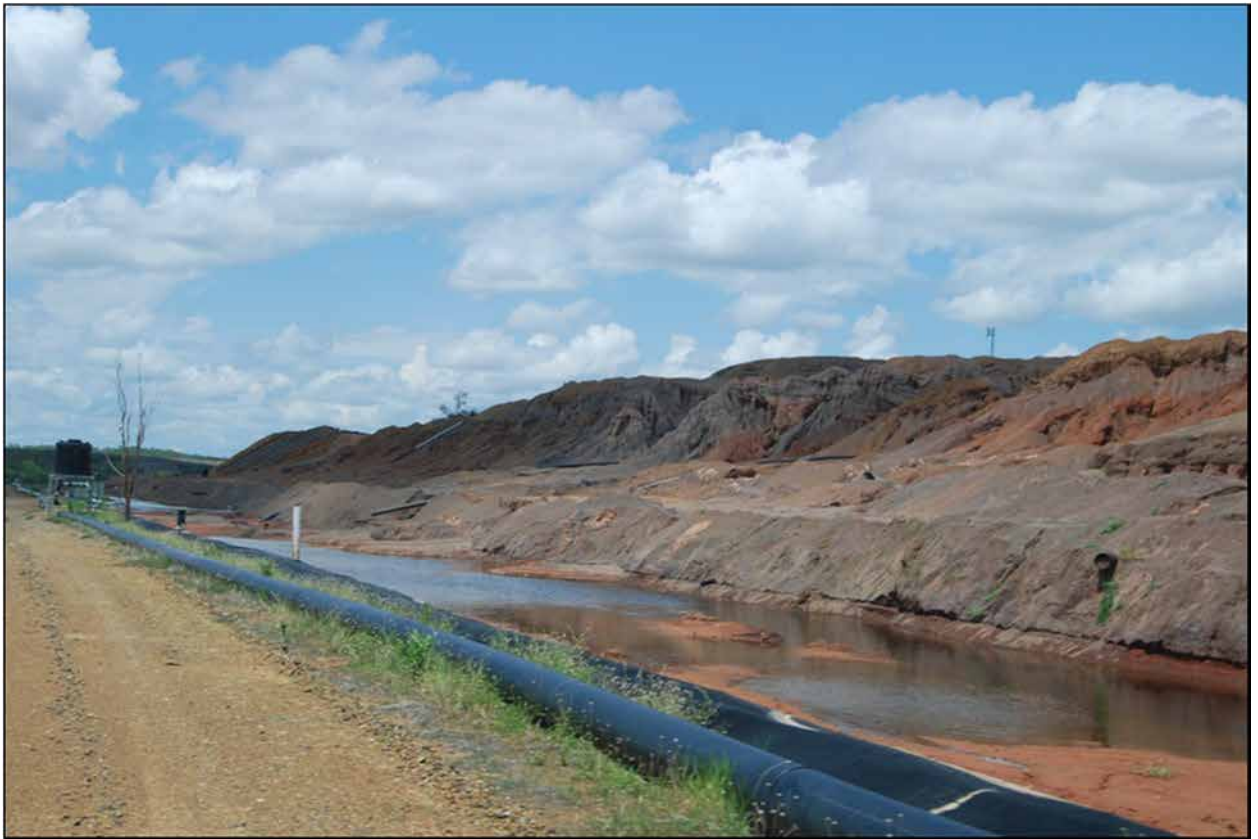
Plate 2-5 Heap Leach Pad
