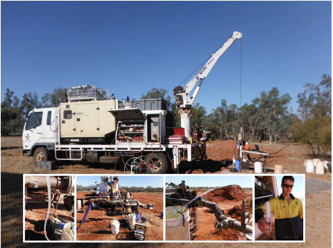
Gas entrapped in Reaphook Paleochannel aquifer being collected during hydraulic pump test on bore RC # 26 (bore site 4A)
