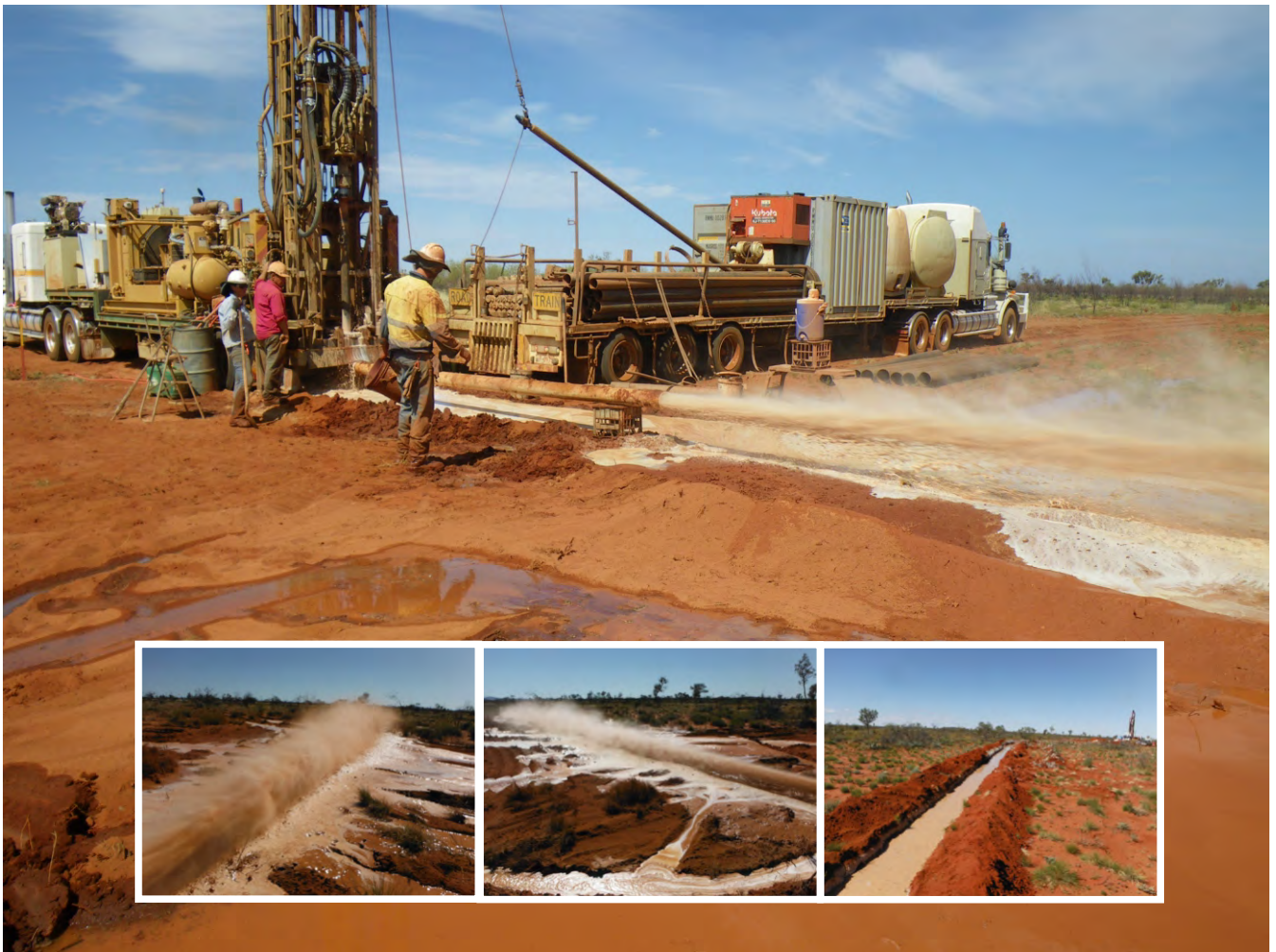
Murrnaji Drillers completed the stage 1 rapid water exploration program using a T3 Drilling Rig and air circulation. The 3 small photos are L2 Drillers drilling bores in the Reaphook Paleochannel
