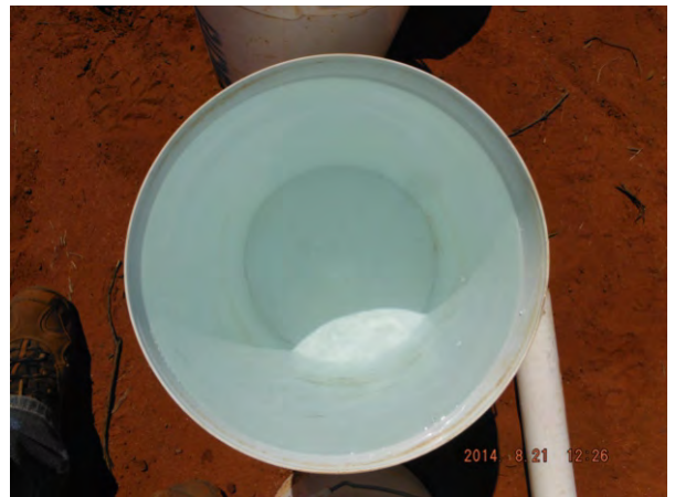
All of the 6 bores tested pumped no sediment over most of the pump testing.
