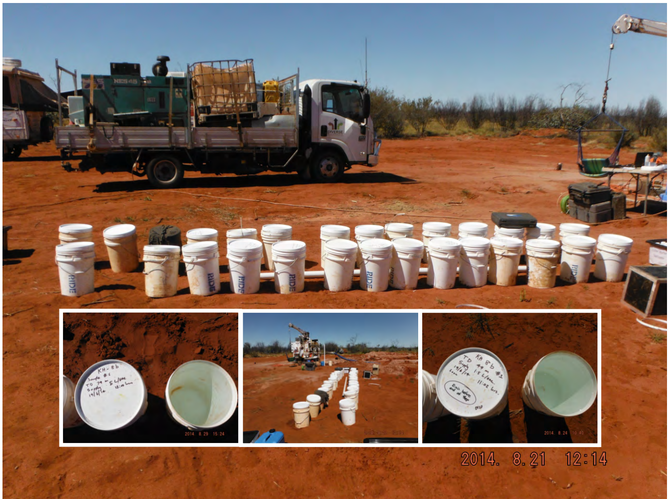
20 L water samples taken during hydraulic pump testing for field water analysis and photographs of sediment pumped during the tests.
