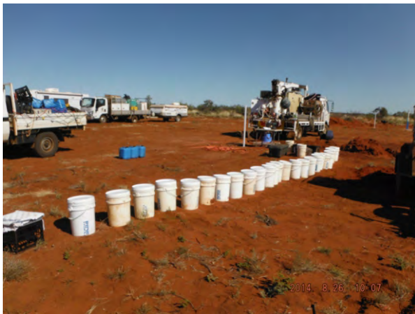
Water samples for field water analysis EC, OH & pH; bore RC # 21 (bore site PB 6)
