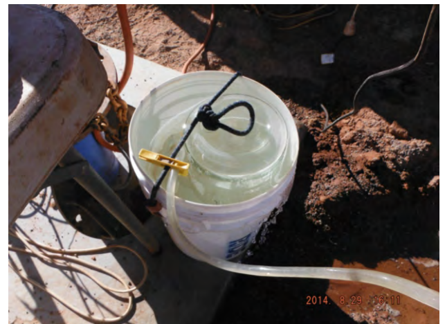
Gas collected in 20 litre glass bottles & sealed for lab analysis
