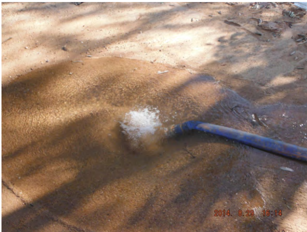
Discharging pumped groundwater into Day Creek from bore RC # 26 (4A) note the gas bubbles
