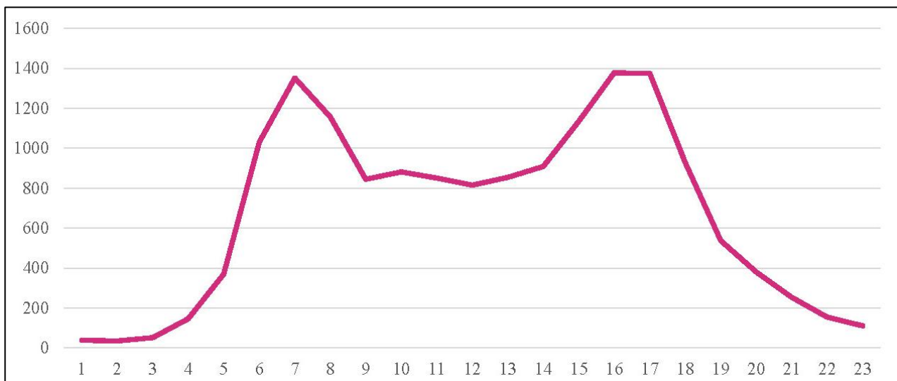
Figure 2-10. Graph of hourly traffic profile over a 24-hour period
