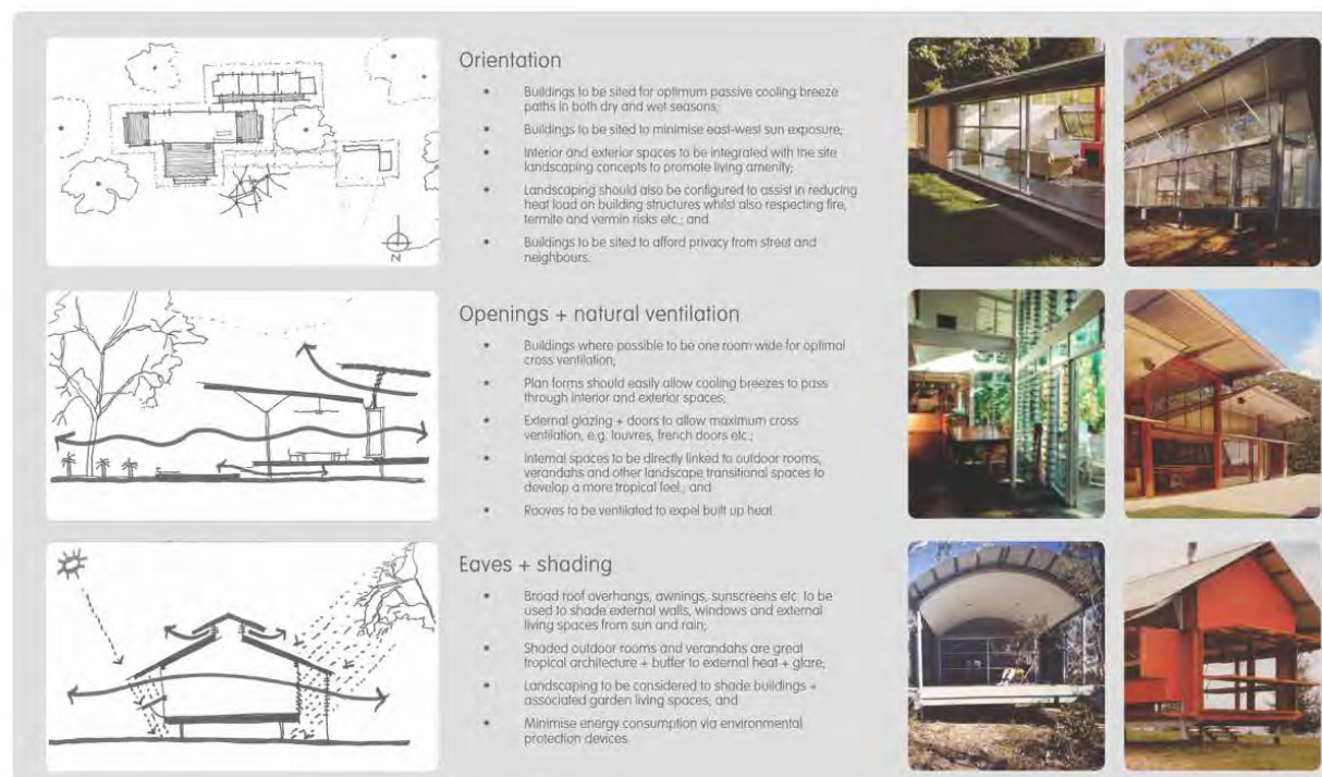
Figure 2.3 Sketches and photographs of the characteristics that will underpin housing design at Noonamah Ridge
