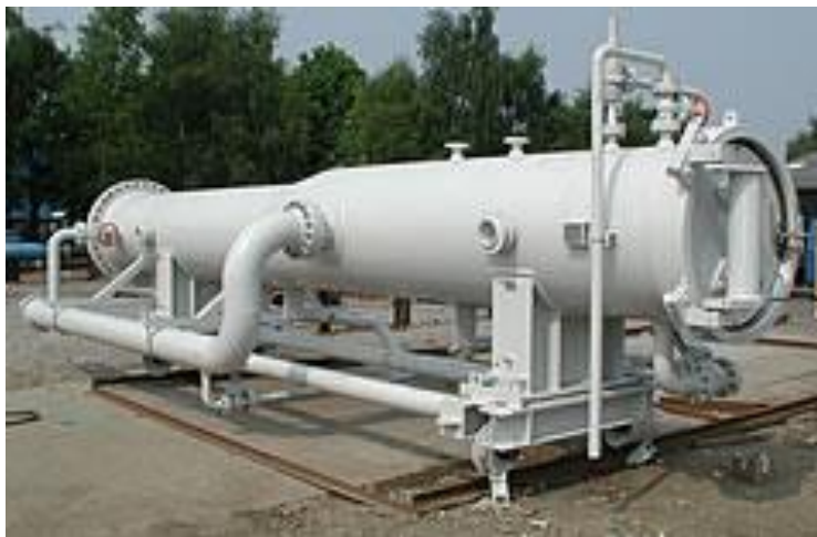
Figure 6: Typical PIG Launcher / Receiver Facility
