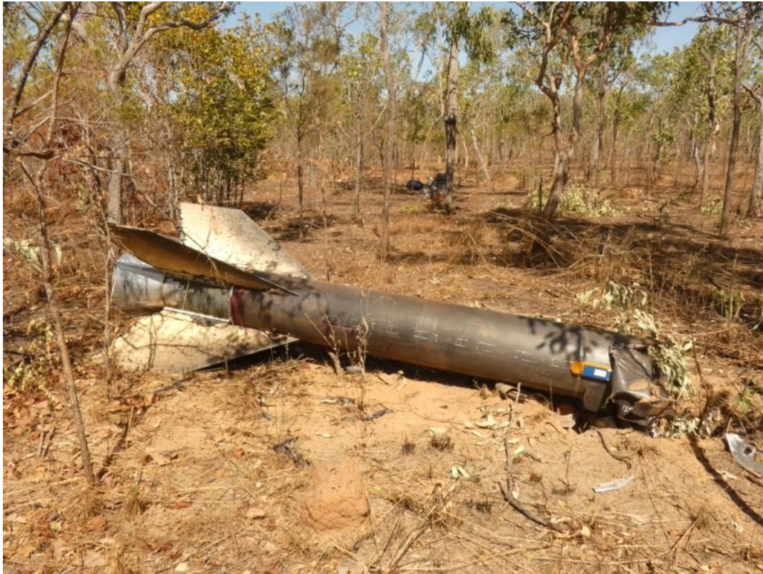
Figure 6 Recovered first stage of BBIX launched from ASC (note lack of damage to vegetation and ground)
