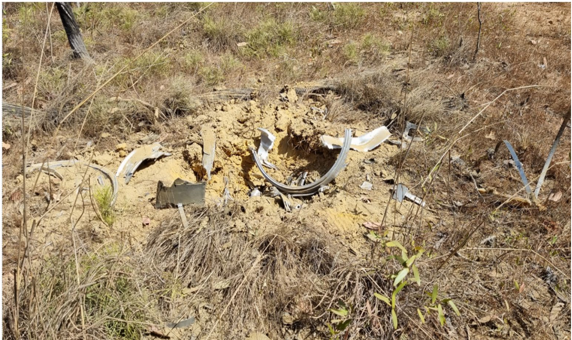
Figure 6: Payload debris from LV (BBIX rocket) recovered on land in East Arnhem Land
