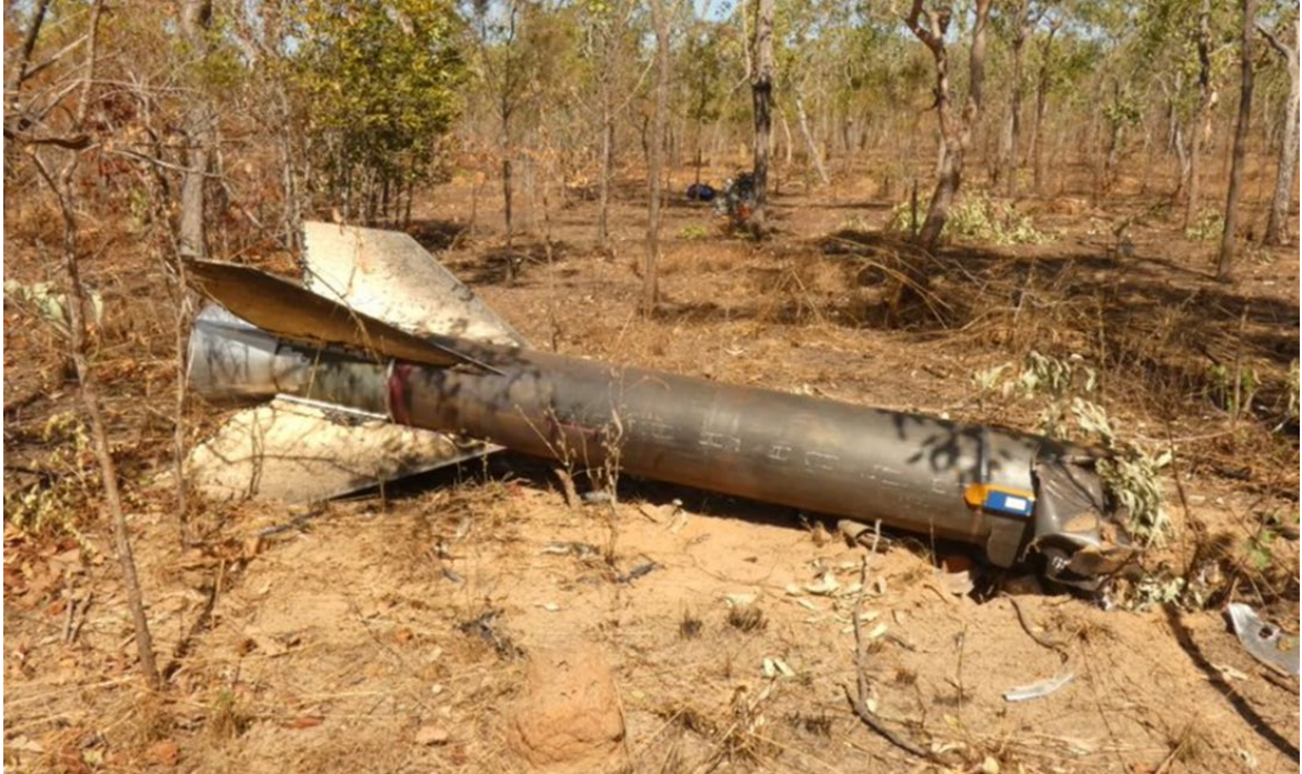
Figure 5: Stage 1 LV (BBIX rocket) recovered on land in East Arnhem Land
