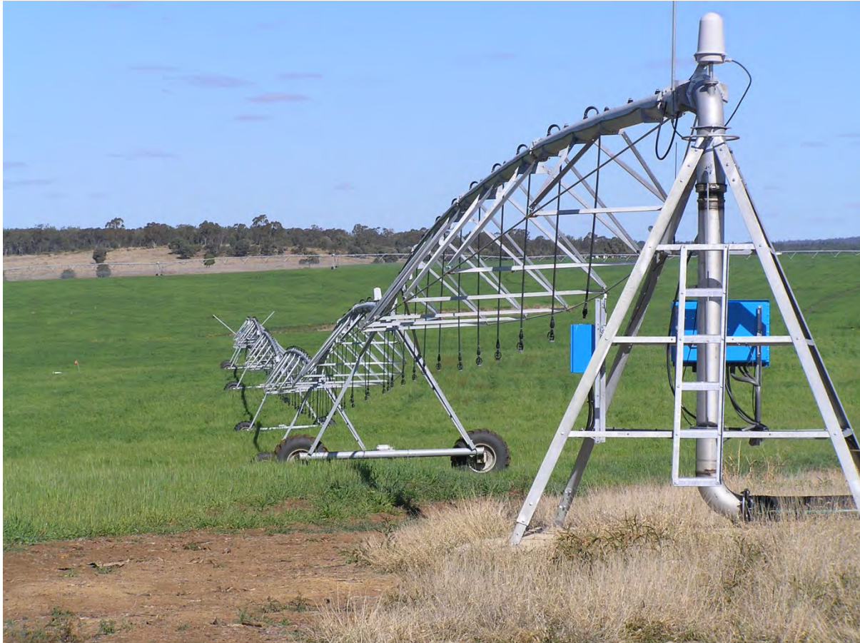
Figure 10-12 An example of a Pivot Irrigation System
