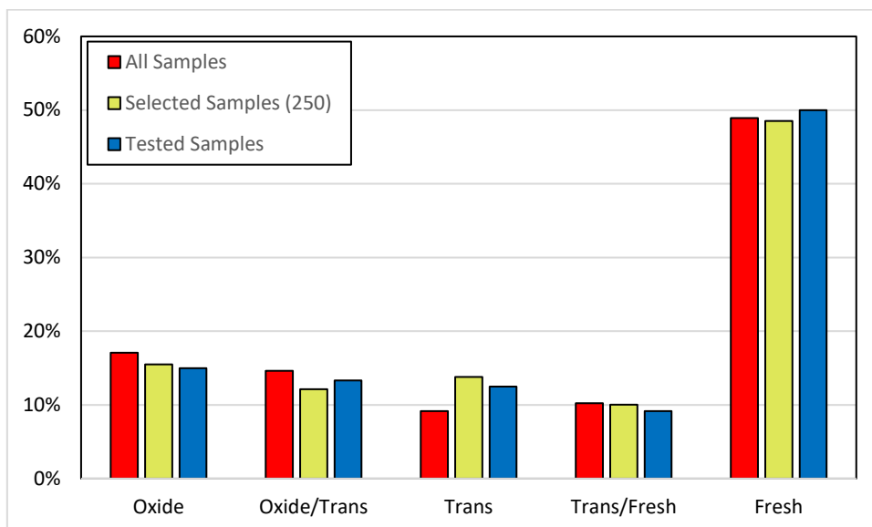
Figure 7: Percent samples from each oxidation state (fully oxidised to fresh) for all samples from the drill holes shown in Figure 5, samples initially selected for testing, and the sub-set of samples which underwent testing.
