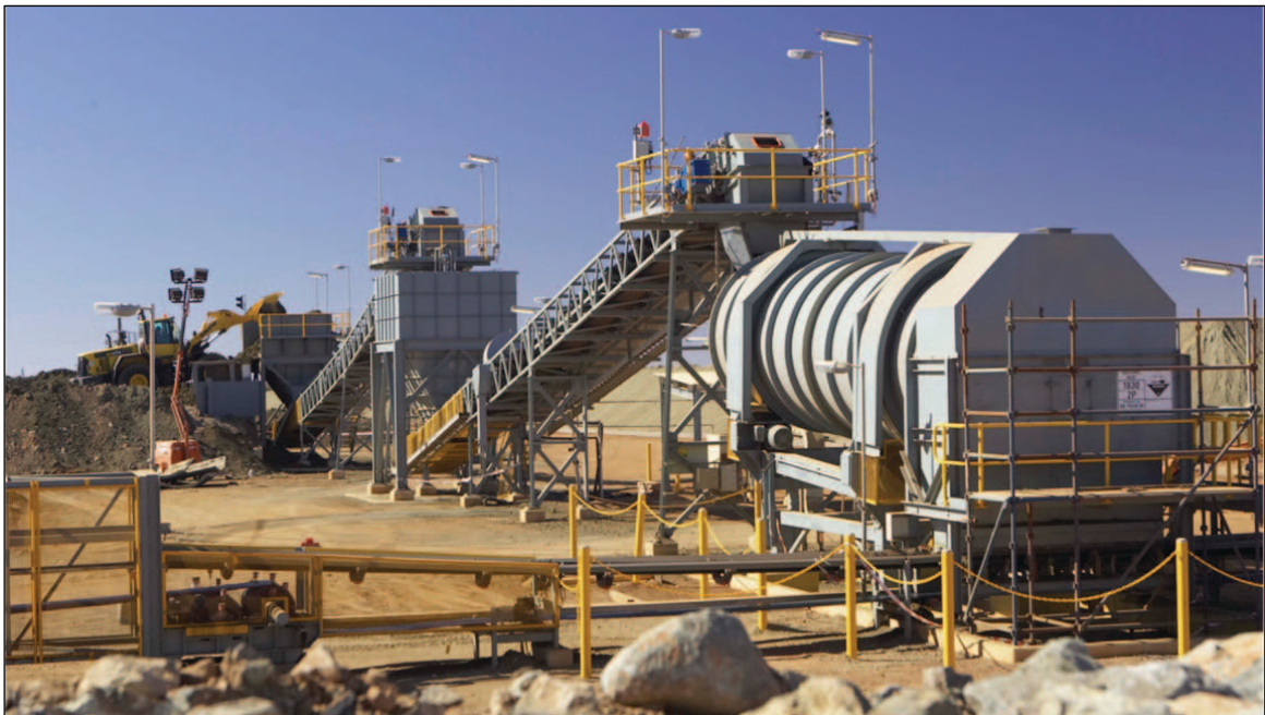
Plate 4.4 – A Typical Agglomeration Circuit and Drum
