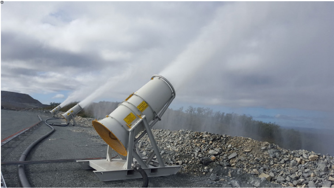
Plate 4.2 – Evaporators in use at Mt Morgan, QLD
