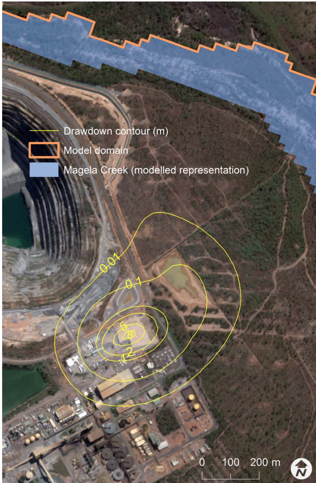
Figure 8-11: Groundwater drawdown at the end of 2020
