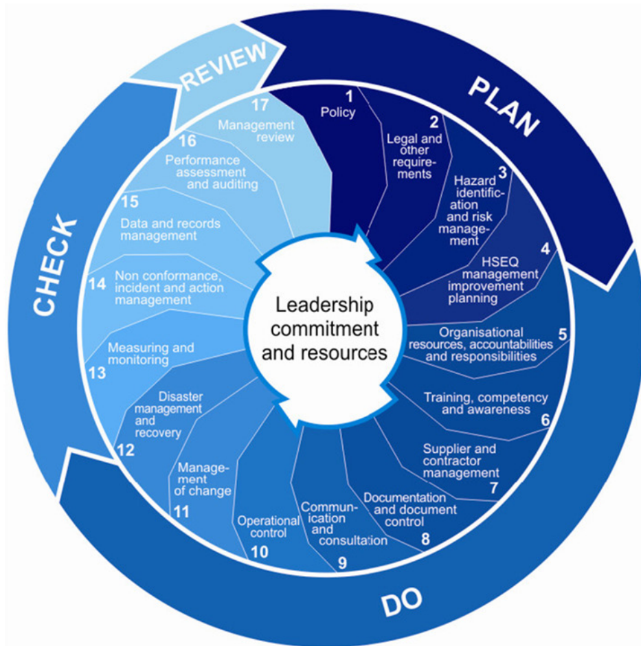
Figure 22: Health, safety and environment management system elements
