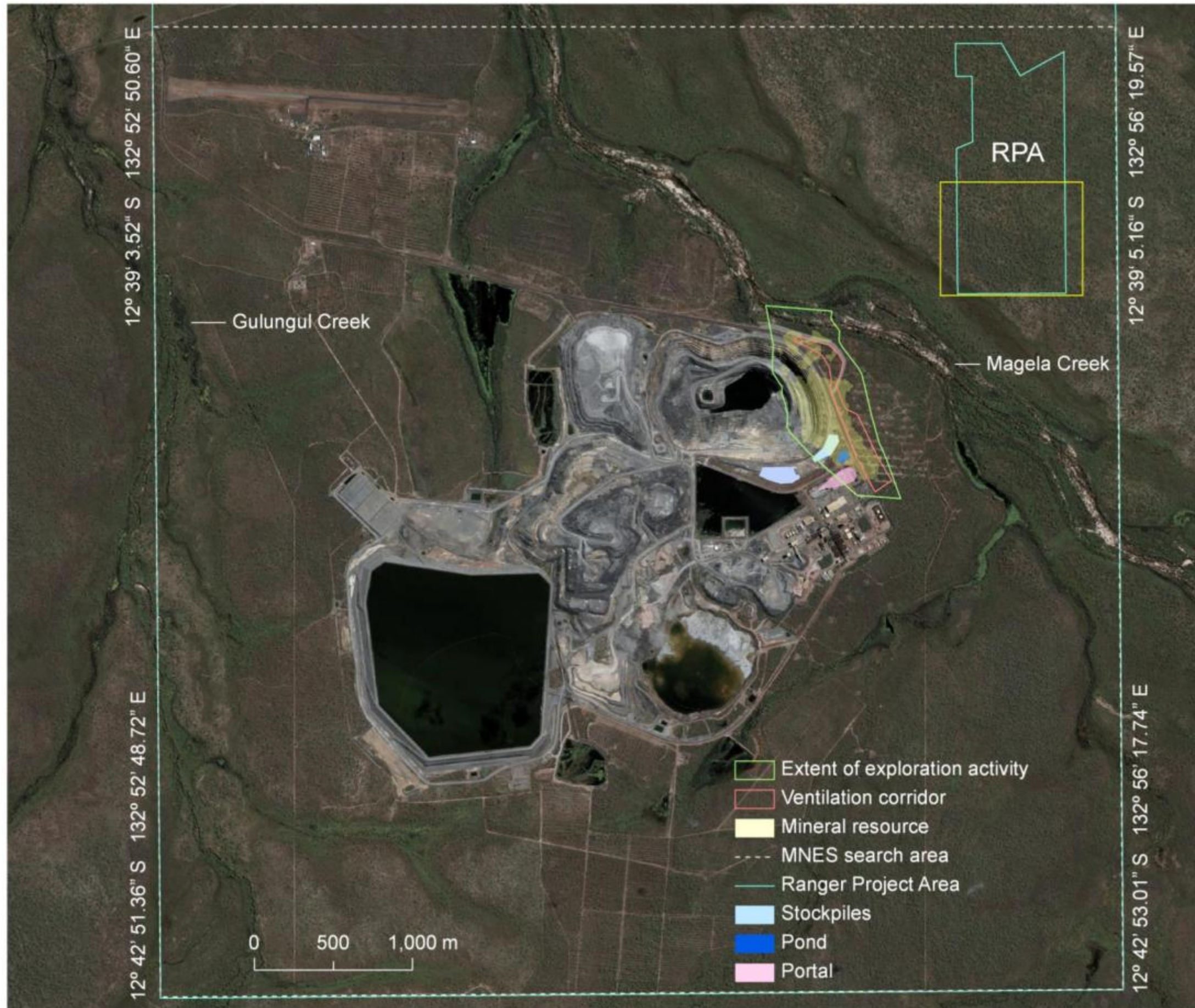
Figure 2: Contextual overview of the Ranger 3 Deeps mineral resource and indicative footprint of key infrastructure within the Ranger Project Area, including matters of national environmental significance (MNES) search coordinates. See Figure 11 for an enlargement of the immediate area of the proposed action. (NB: stockpiles, pond and portal are existing infrastructure constructed for the Ranger 3 Deeps Exploration Decline project.)
