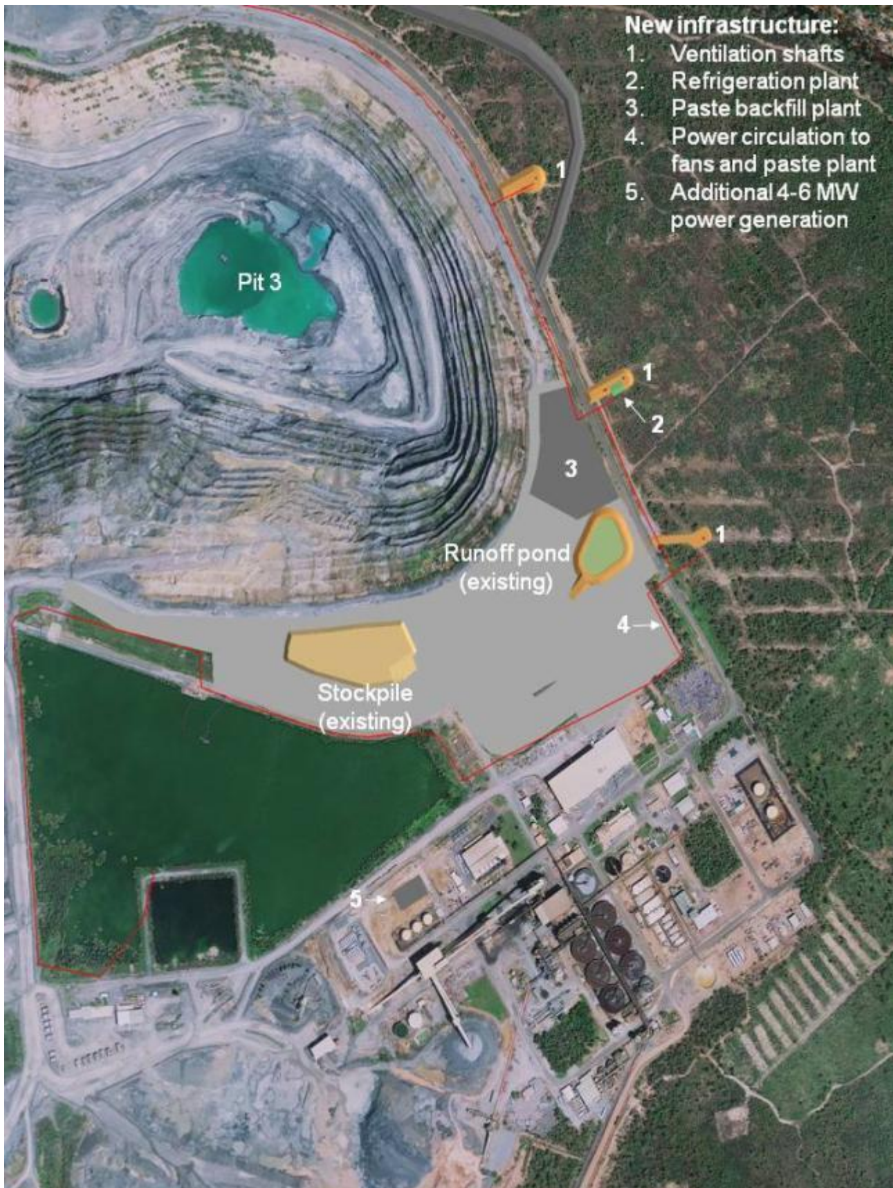
Figure 3: Indicative location of the proposed action infrastructure in relation to existing infrastructure
