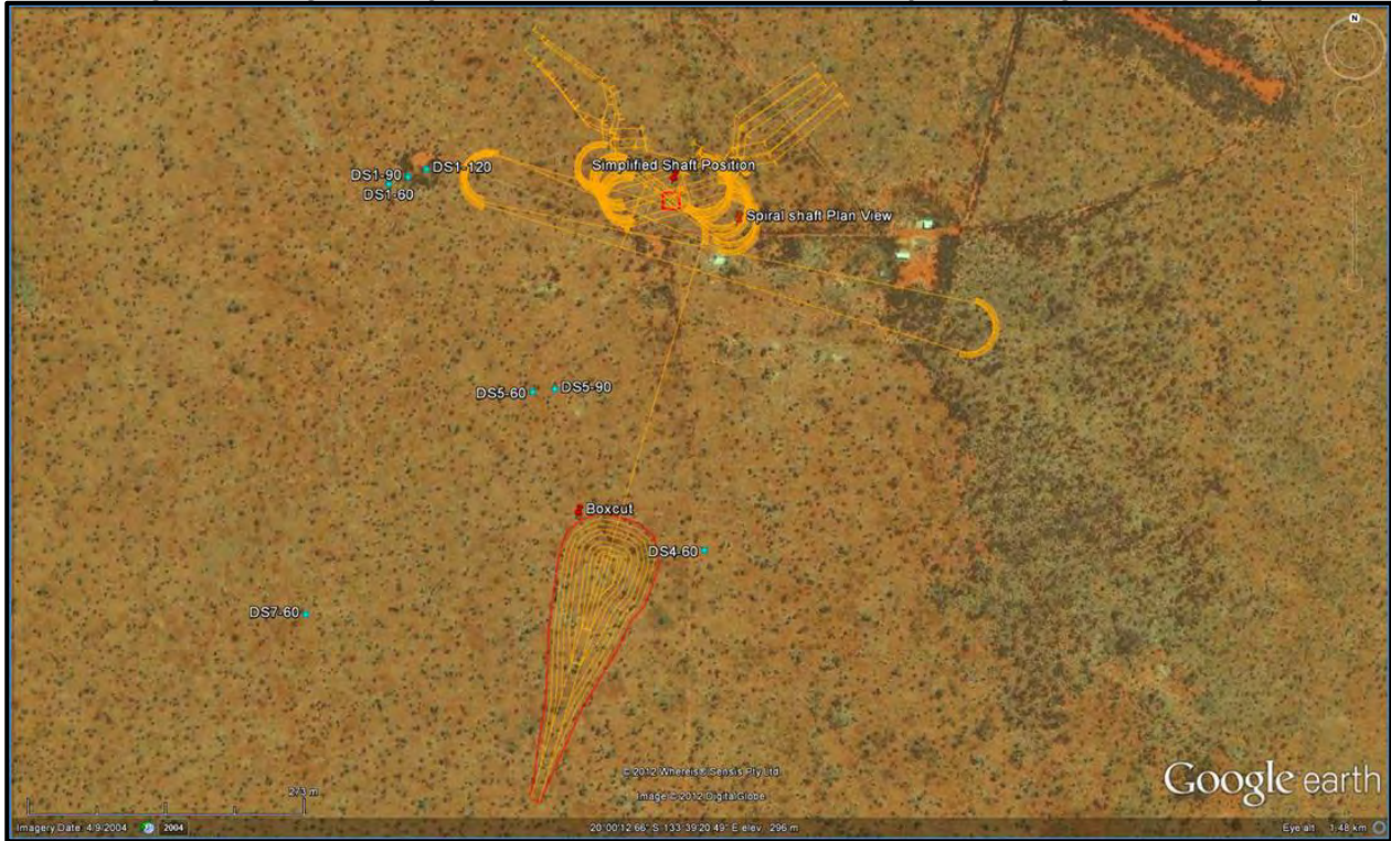
Figure 18: Simplified Layout of Proposed Box Cut (30m deep) and Decline (Google Earth, 2012).
